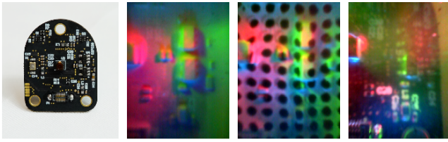
Fig. 28. Effect of different types of elastomers on a DIGIT sensor, the three different types chosen here (left to right) are reflective, reflective with markers and transparent [11]
