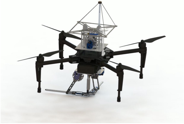
Fig. 15. The SpiderMAV drone which shoots threaded anchors into fixed structures, allowing it to perch[19]
