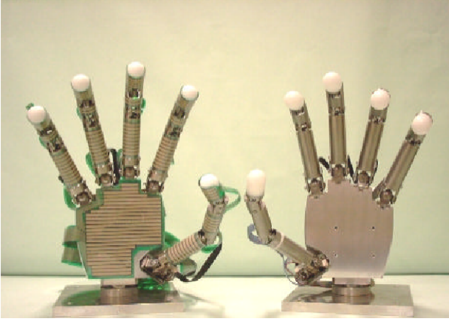
Fig. 17. The Gifu Hand 2, an early demonstration of the benefit of tactile sensing in robotics, it utilizes six-axis fingerprint sensors while also containing a distributed tactile sensing system over the rest of its surface [30]
