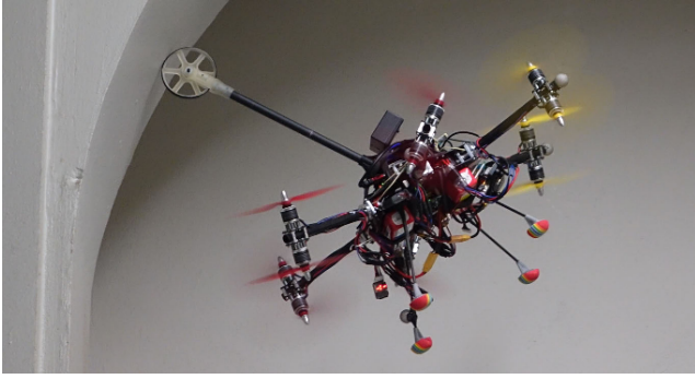
Fig. 8. A Contact-based Inspection Drone demonstrating a use case for aerial manipulators, uses a fully actuated tilt-rotor system [6]
