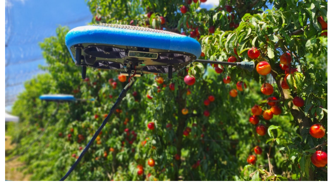
Fig. 10. A precision Agriculture Drone shows yet another use case for aerial manipulators, fruit harvesting [13]
