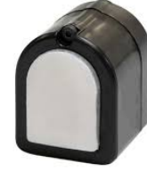
Fig. 7. The DIGIT sensor to be used in the new drone design, it will replace the existing capacitive tactile sensors [12]
