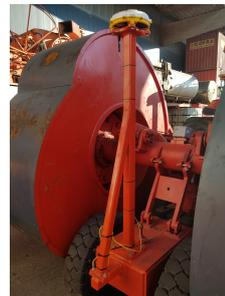
Figure 5.2: Accelerometer location on the centre of the drum axis
