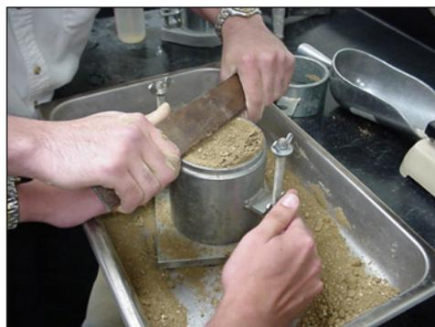
Figure 3.11: Standard proctor test procedure
