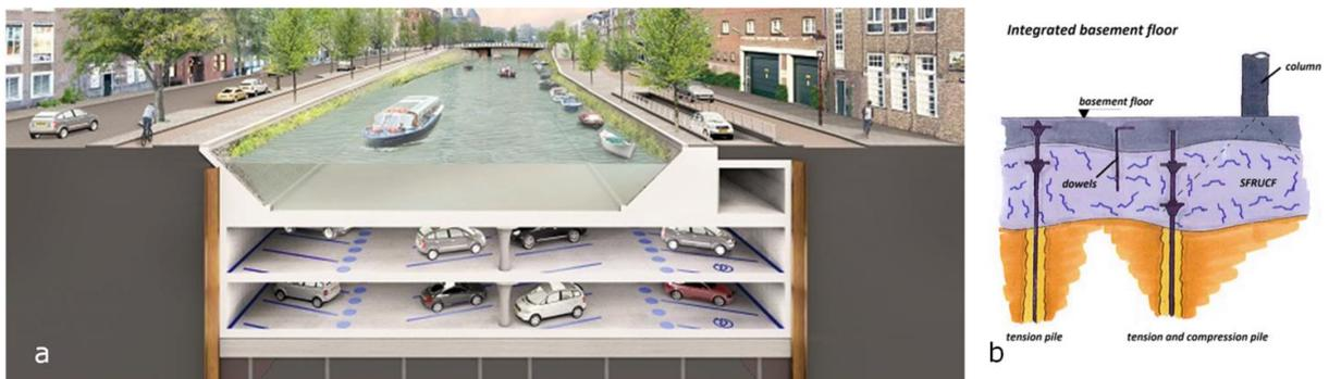
Figure 13 a) Cross-section of the Albert Cuyppgarage (ABT, 2016) b) sketch of the Integrated floor system (ABT, 2016)
