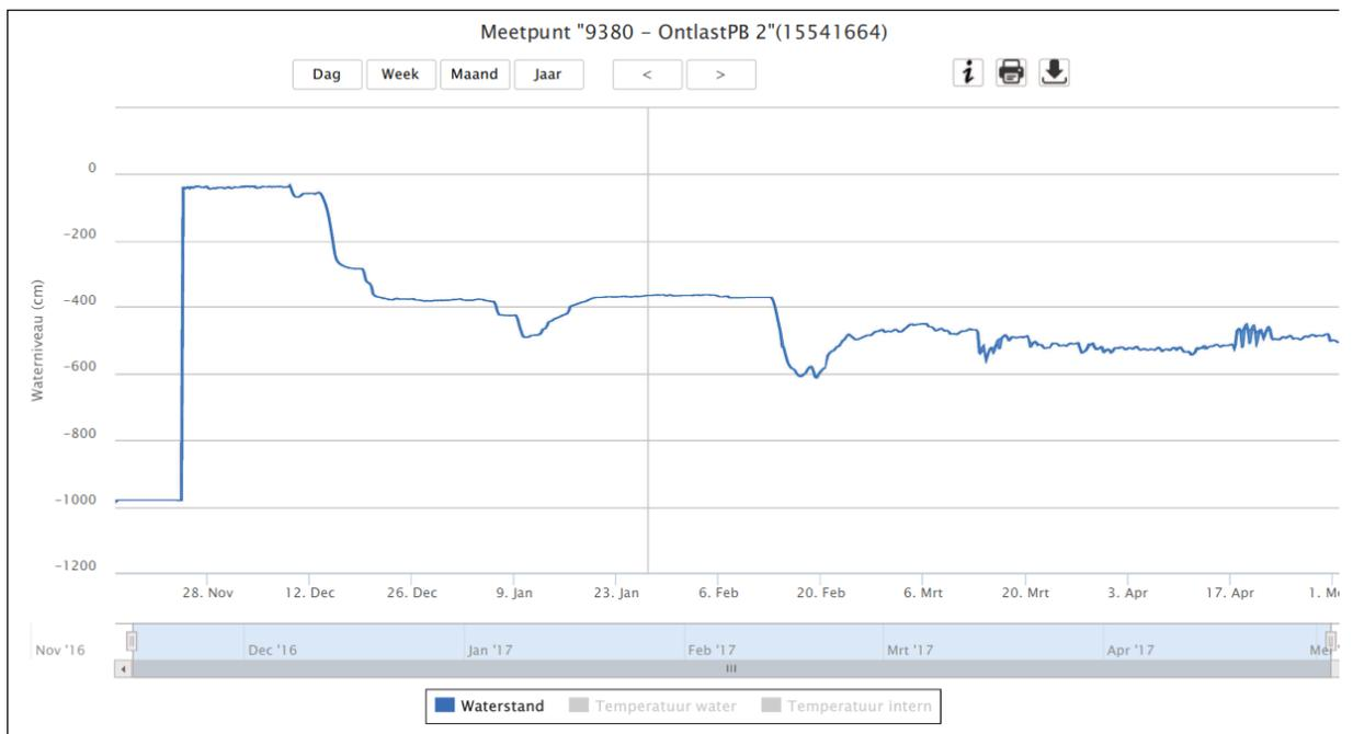
figure B 1 Pressure relief pipe 9380 (Max Bögl, 2016)
