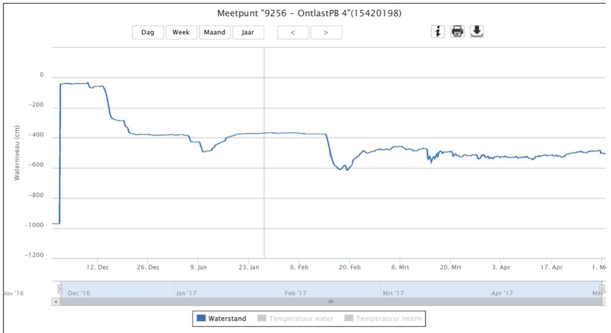
figure B 4 Pressure relief pipe 9256 (Max Bögl, 2016)
