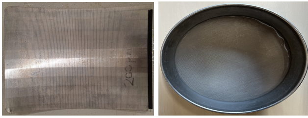
(a) Curved Sieve (200 \mu\text{m} ) (b) Circular Filter (200 \mu\text{m} and 250 \mu\text{m} )
