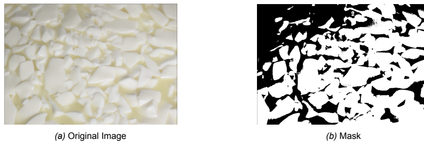
Figure 3.6: K-means segmentation for k = 2
