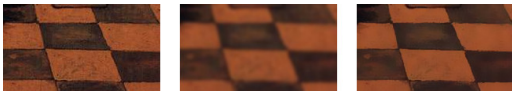
Figure 3: From left to right: detail from original image (Figure 9); Gaussian filtering; Bilateral filtering
