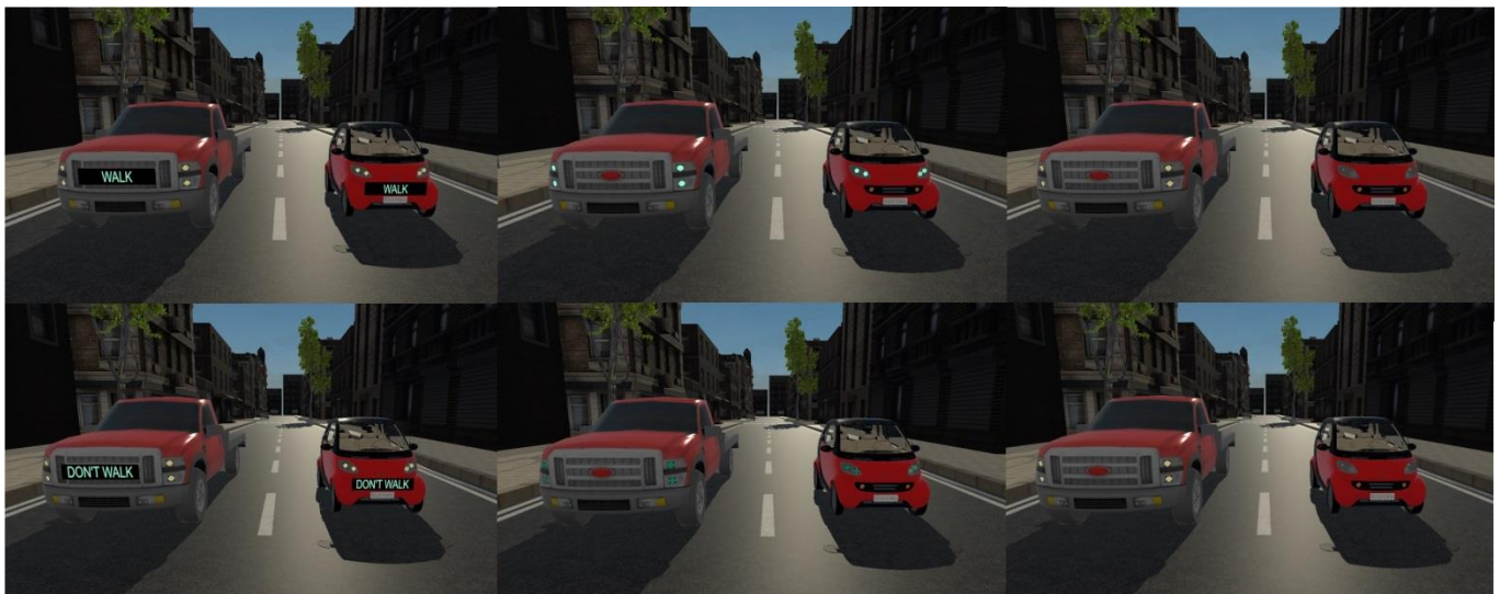
Figure 6: External appearance of the cars used in this simulation. From left to right, top to bottom: Truck Text eHMI Yielding, Smart Text eHMI Yielding, Truck Frontal Braking Lights Yielding, Smart Frontal Braking Lights Yielding, Truck No eHMI Yielding, Smart No eHMI Yielding, Truck Text eHMI Non-Yielding, Smart Text eHMI Non-Yielding, Truck Frontal Braking Lights Non-Yielding, Smart Frontal Braking Lights Non-Yielding, Truck No eHMI Non-Yielding, Smart No eHMI Non-Yielding
