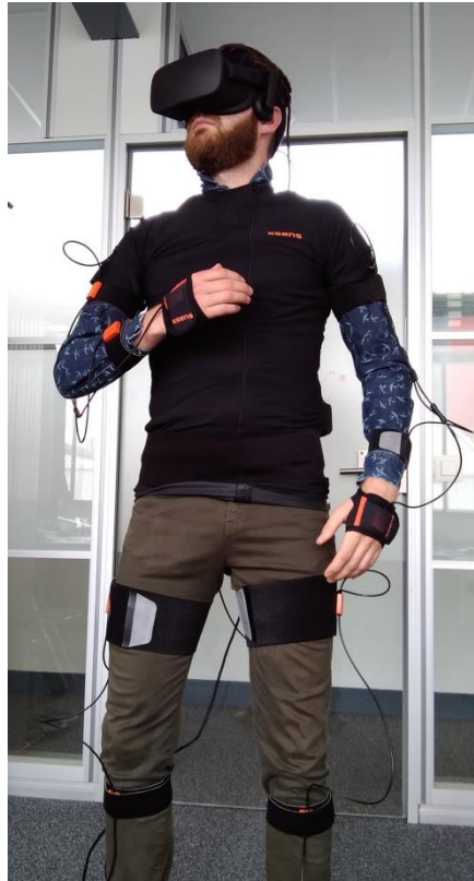
Figure 23: Xsens and Oculus Set-up
