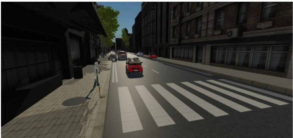
Figure 2: Cars approaching participant in the VR Environment. The starting location of the participant during the experiment is visible here as the grey circle behind the blue leg of the avatar. Cars only approached the participants from their left-hand side. Participants were able to cross the road up until the third zebra stripe counting from the curb.
