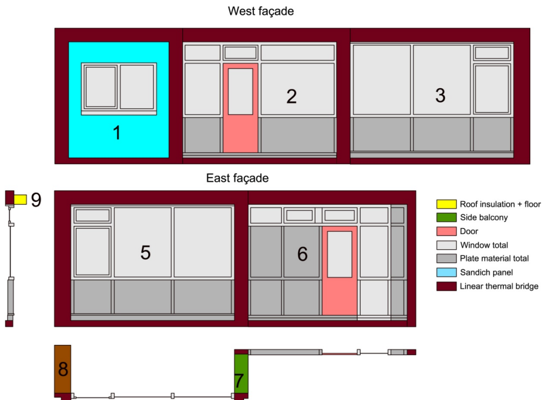
Figure 4-43: Simplified current façade for the EPC calculation
