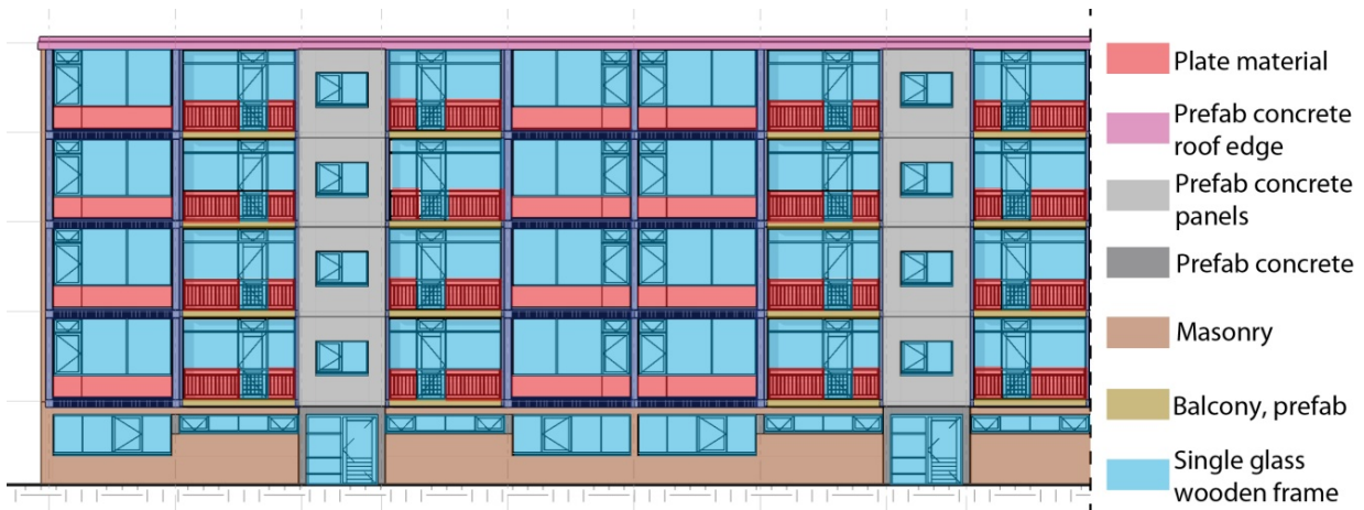
Figure 4-23: Part of the front/west façade of the portiekflat analyzed in façade materials
