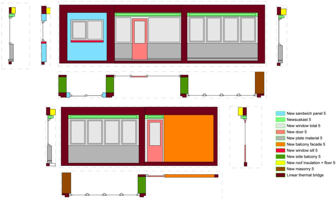
Figure F- 18: Design for strategy 3, interior upgrading, simplified for EPC calculations
