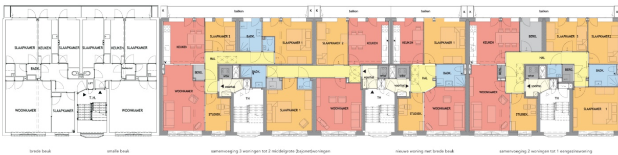
Figure 2-27: Floor plan before refurbishment (left) and after refurbishment (apartments in colour to the right) (Archivolt Architecten bv, 2012)
