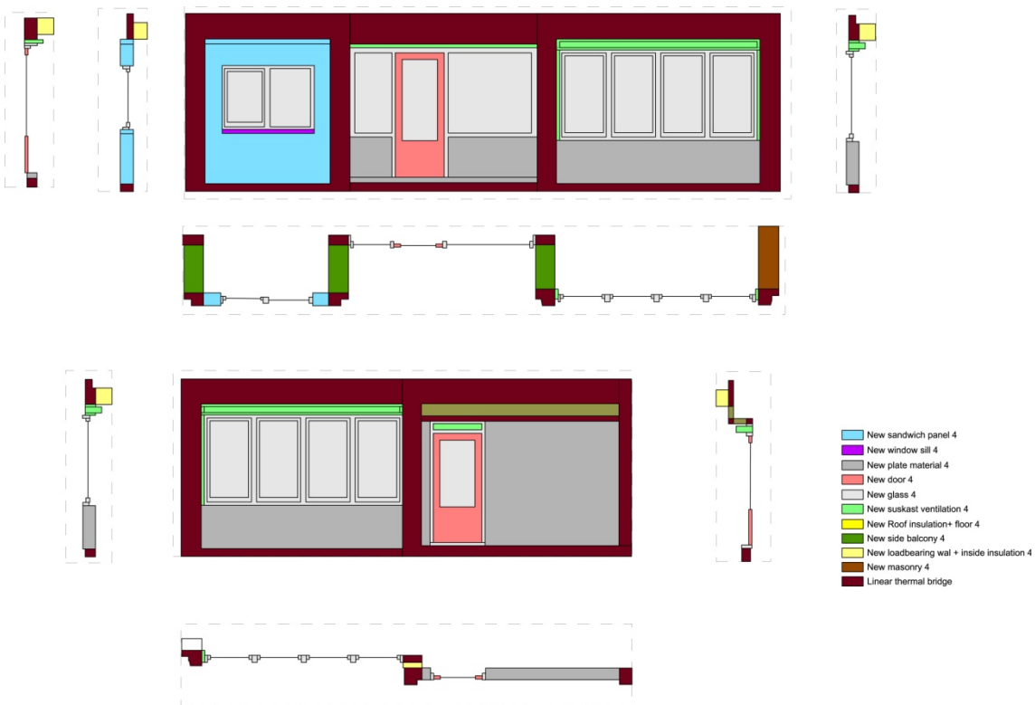
Figure F- 24: Design for strategy 5, simplified for EPC calculations
