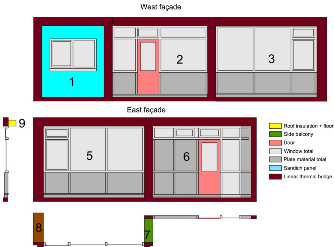
Figure F- 2: Current façade, simplified for EPC calculations
