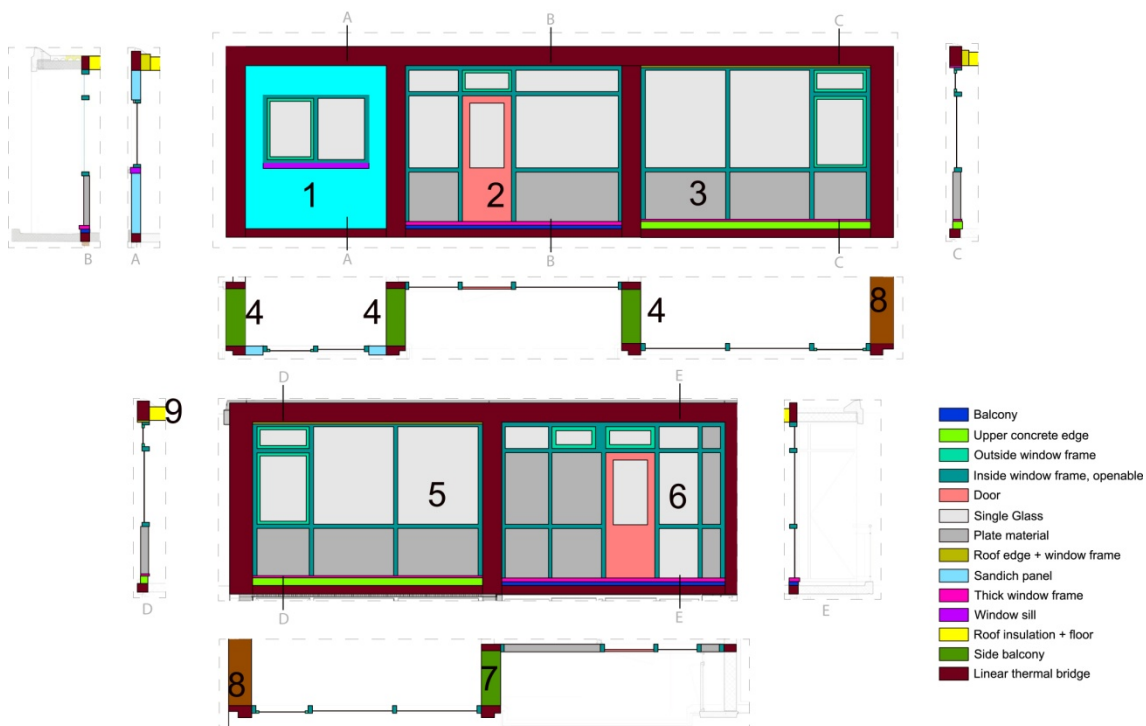
Figure F- 1: Current façade, with façade components
