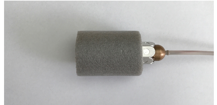
Fig. 34: Assembled prototype without 3D textures inside a short piece of the isolation tube.
