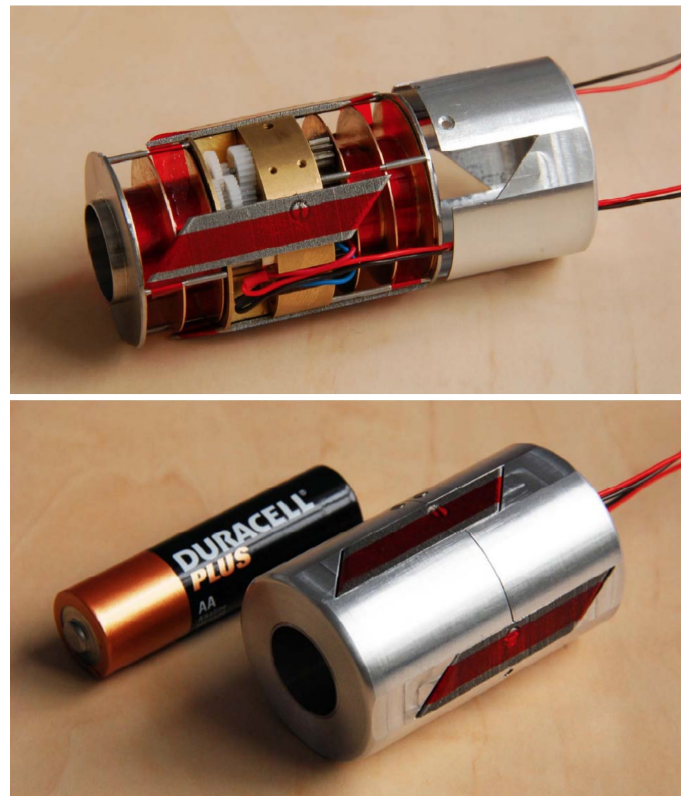
Fig. 5: Two pictures of a device that can pull a colonoscope through the colon using mucoadhesive films. The top picture shows the inside of the device where the tape is stored and motors and transmission are housed. The bottom picture shows the full device compared to an AA battery.
