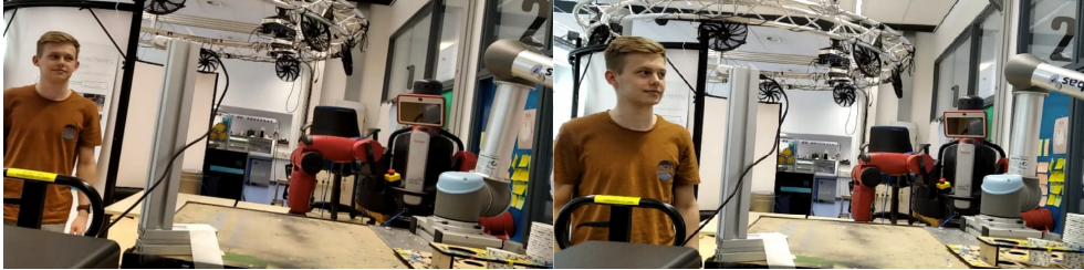
Figure 5.11: Safety Slowdown demo, as person approaches robot at work, its task velocity will be dynamically linked to operator's position relative to robot
