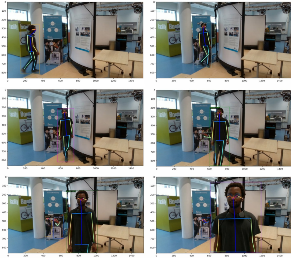
Figure 5.12: Safety Track where a person’s skeleton is tracked through 3D space around the robot
