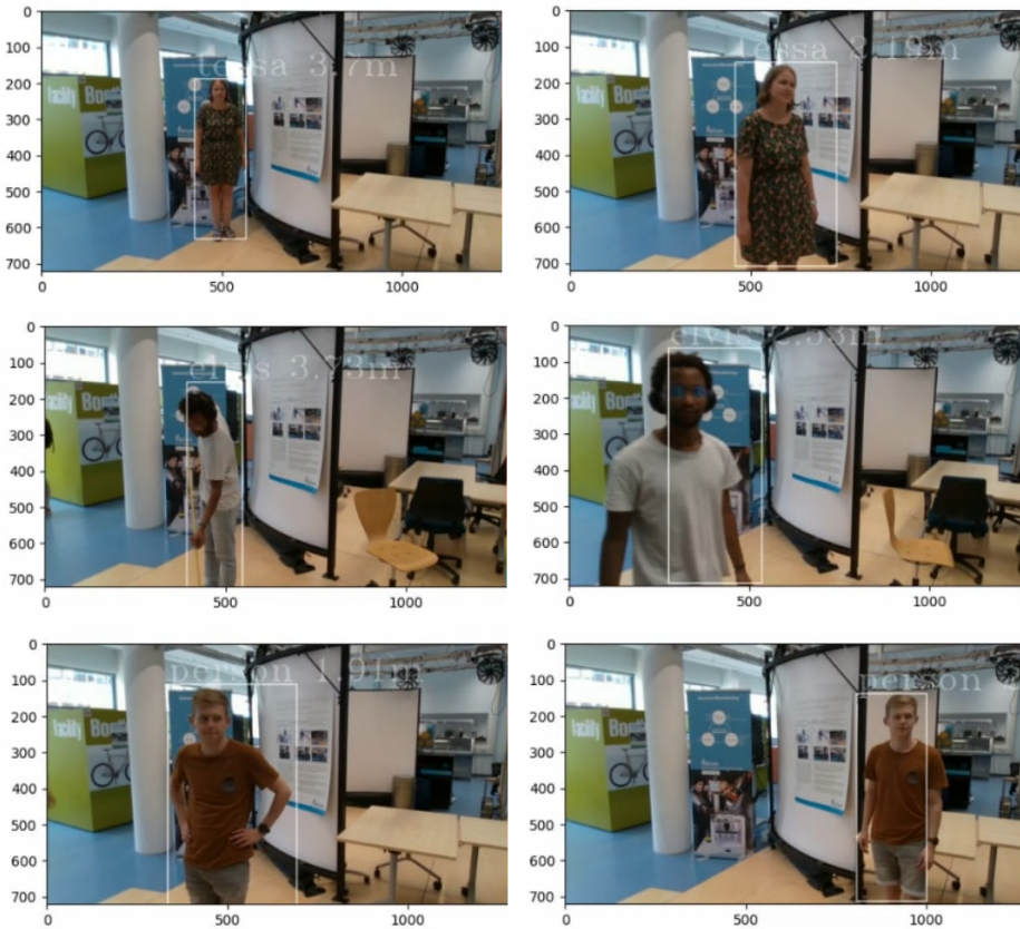
Figure 5.5: Examples of MobileNet detections, with corner cases on the right (either incomplete or non-tight bounding boxes)
