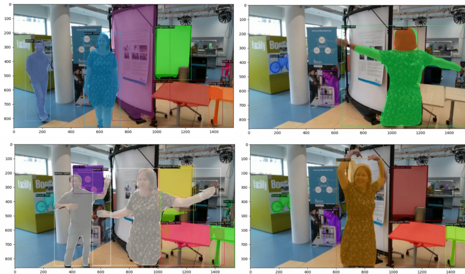
Figure 5.6: Examples of R-CNN detections, with corner cases on the right (either incomplete segmentations or low confidence results)
