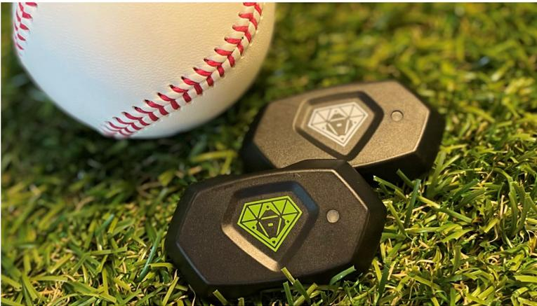
Figure 3.1.: Pitch Perfect sensor system for measuring pelvis and trunk kinematics and separation time between them.
