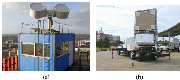
Fig. 2. Photos of polarimetric weather radars: (a) MESEWI: X-band mechanically scanning radar operated by TU Delft. (b) HORUS PPAR by the Advanced Radar Research Center [2]. Licensed under CC BY 4.0.
