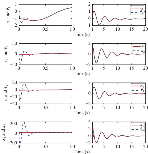
Fig. 6. System response and ESO output.
