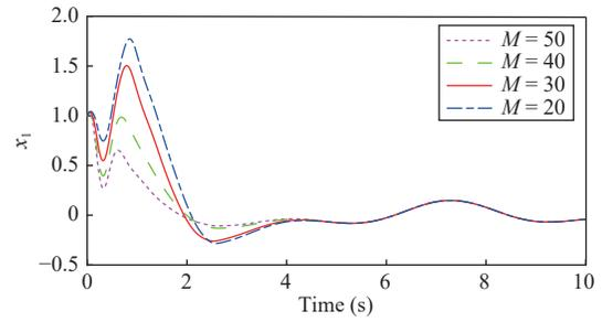
Fig. 5. System response under different saturation bounds.
