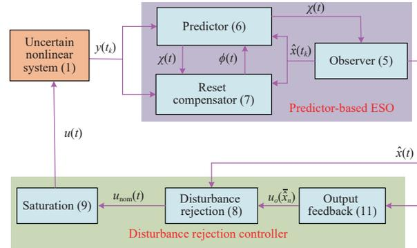
Fig. 1. The architecture of the proposed ESO and the disturbance rejection controller.
