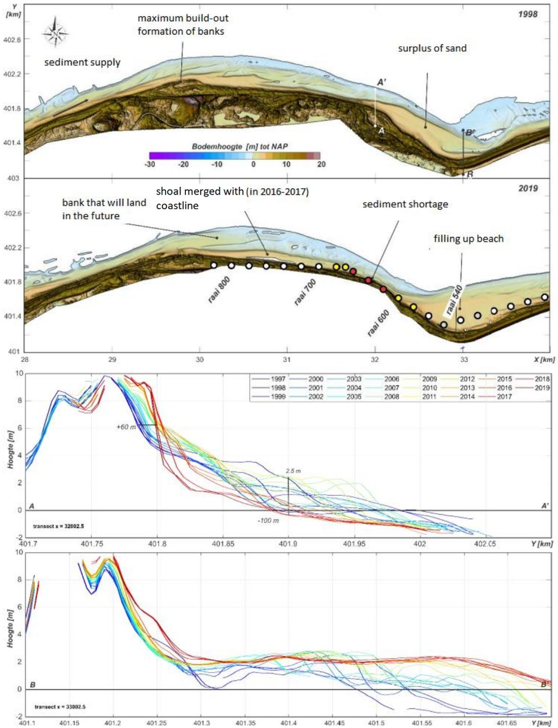
Figure 2.6: Overview from LiDAR measurements for 1998 and 2019 (top two images), and the development the bottom height in crosssections A-A' and B-B' (bottom two images). (Elias & Quataert, 2021)
