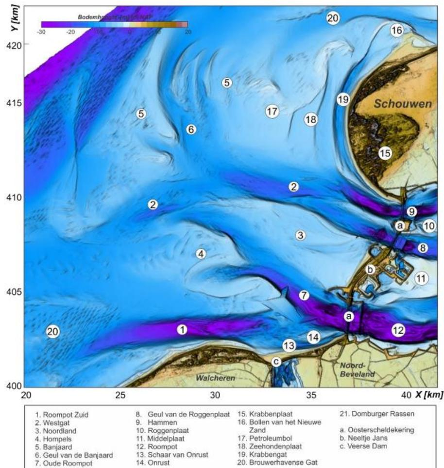
Figure 1.2: An overview of the channels and shoals of the Eastern Scheldt ebb-tidal delta based on the 2019 Vakloding (Elias & Quataert, 2021)
