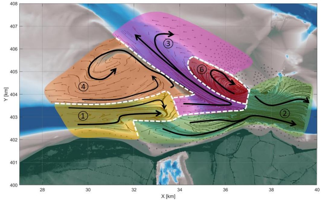
Figure 5.6: 1988 bathymetry with barrier. The dotted white lines indicate boundaries between divergent or non-convergent parallel paths. The black arrows indicate the main sediment pathways.
