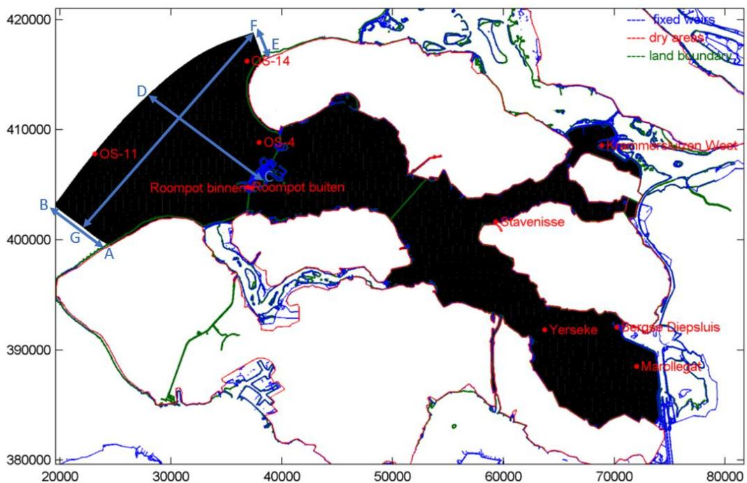
Figure 4.1: Overview the D-HYDRO Eastern Scheldt network with the locations of the waterlevel measuring stations. Distances: A-B = 6km, C-D = 13km, E-F = 3km and F-G = 23km. (Tiessen et al., 2019).
