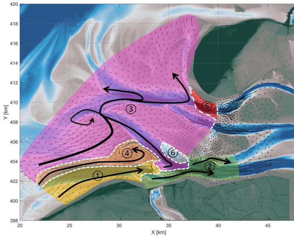
Figure 5.2: 1988 bathymetry with barrier. The dotted white lines indicate boundaries between divergent or non-convergent parallel paths. The black arrows indicate the main sediment pathways.
