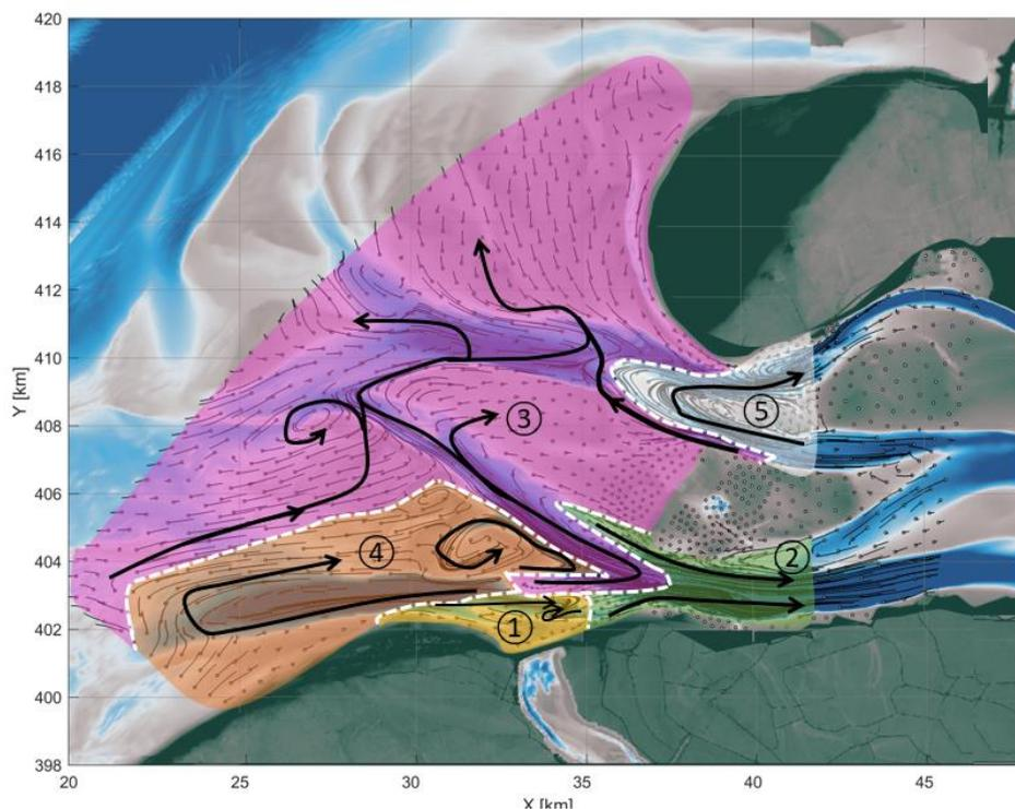
Figure 5.1: 1976 bathymetry without barrier. The dotted white lines indicate boundaries between divergent or non-convergent parallel paths. The black arrows indicate the main sediment pathways.
