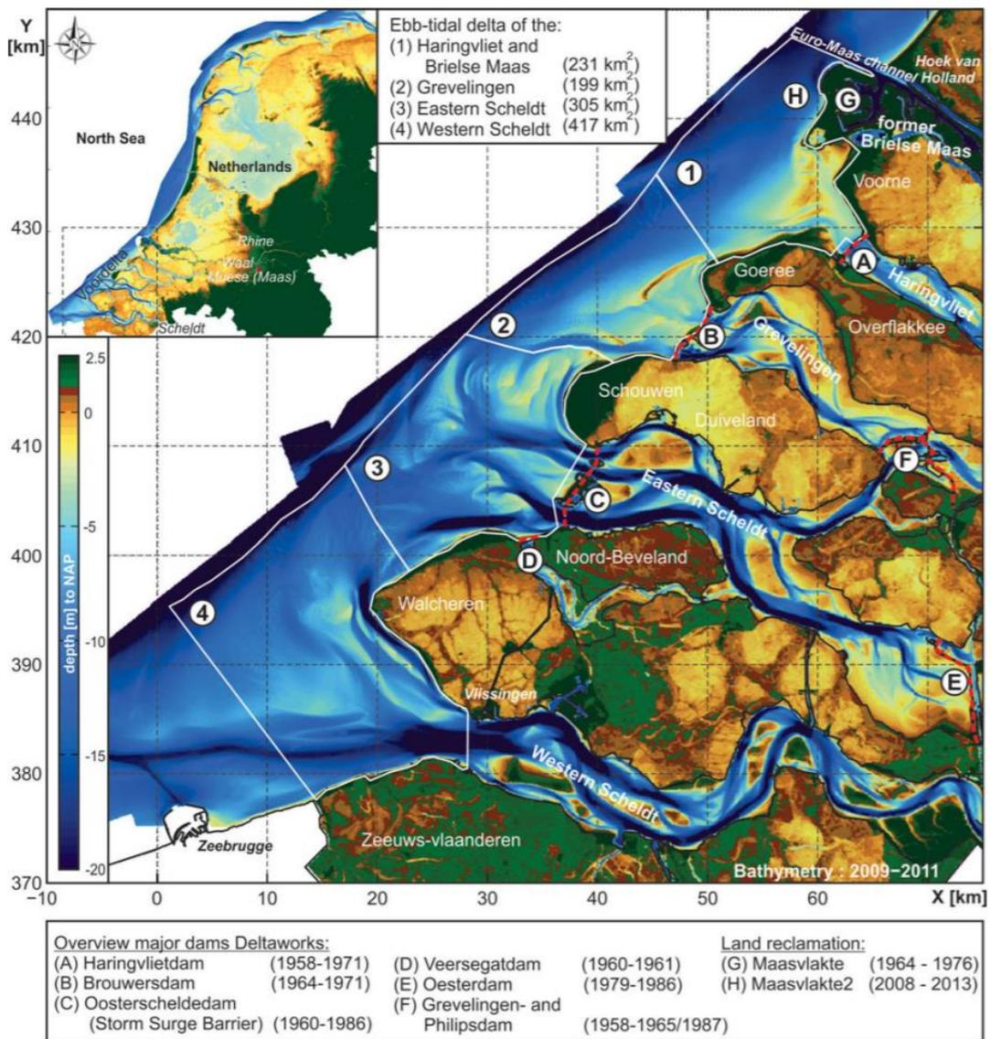
Figure 1.1: Overview of the Dutch Delta, the estuaries which form the Voordelta. The red dashed lines indicate the major dams constructed as part of the Delta Plan. The white lines are an indication of the boundaries of the ebb-tidal deltas of the respective estuaries. Depths are given in m relative to NAP (Normaal Amsterdams Peil), the Dutch ordnance datum which is about present-day mean sea level (MSL). Elias et al., (2017).
