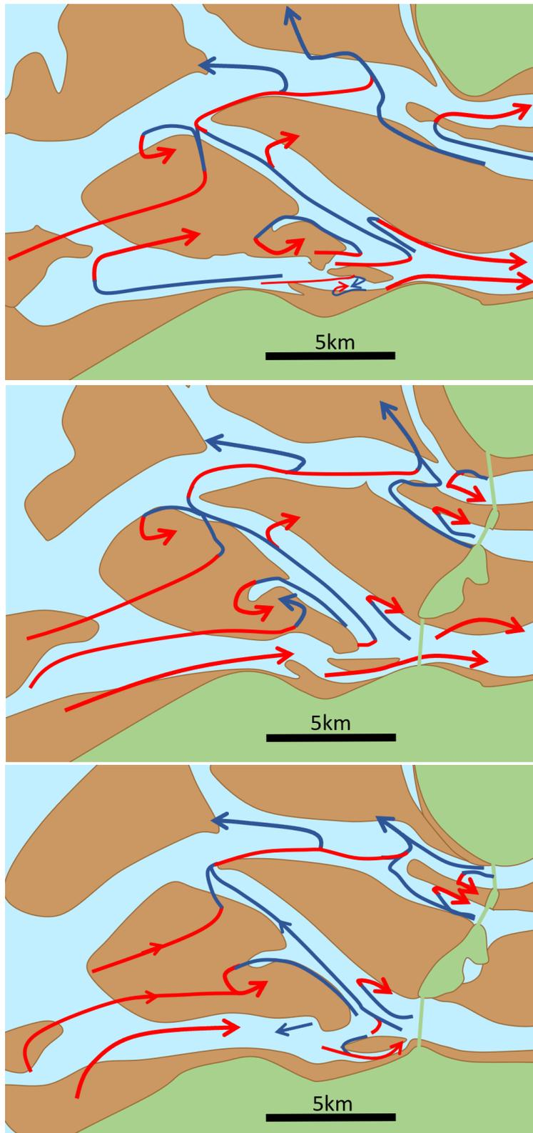
Figure 6.1: Schematization of the main ebb- and flood-dominant sediment transport trajectories in 1976 (top), 1988 (middle) and 2019 (bottom). The red and blue arrows indicate flood- and ebb-dominant transport pathways respectively.
