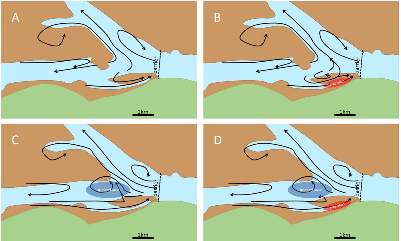
Figure 6.4: Schematization of the main sediment trajectories in different scenarios. A represents the sediment trajectories with the original 2019 bathymetry. B represents the sediment trajectories with a nourishment in the Schaar van Orrust. C represents the sediment trajectories with the removal of sediment from the Roompot-Hompels connection. D represents the sediment trajectories with both the nourishment and the removal of sediment.
