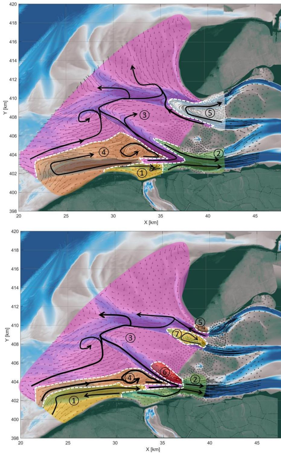
Figure 5.4: Top: 1976 bathymetry without barrier. Bottom: 1976 bathymetry with barrier. The dotted white lines indicate boundaries between divergent or non-convergent parallel paths. The black arrows indicate the main sediment pathways.
