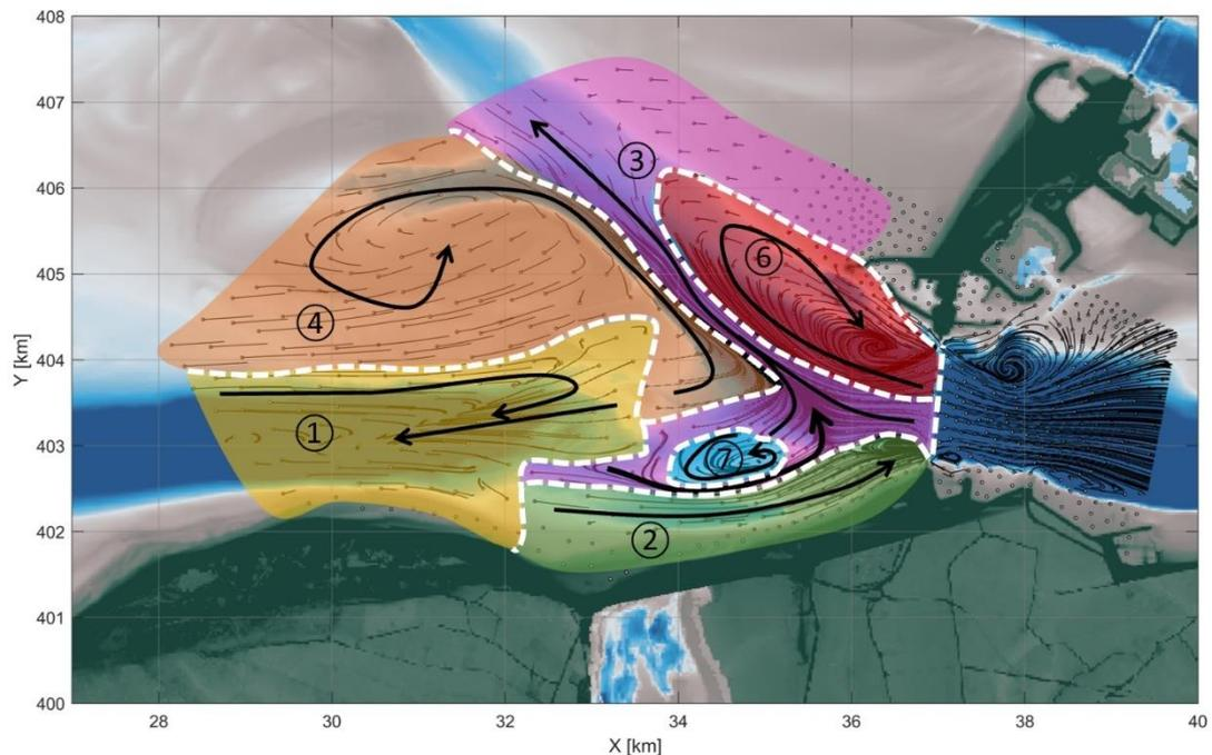
Figure 5.8: 2019 bathymetry with the implemented nourishment zoomed in on the Roompot channel. The dotted white lines indicate boundaries between divergent or non-convergent parallel paths. The black arrows indicate the main sediment pathways.
