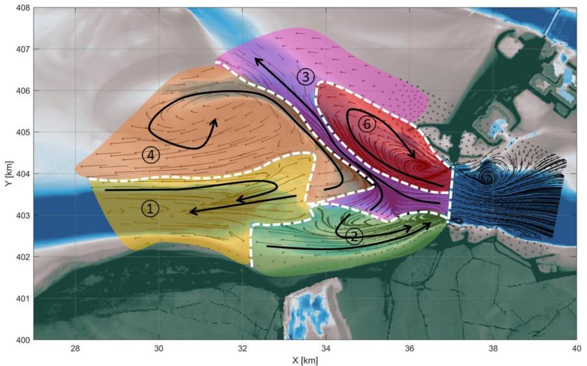
Figure 5.7: 2019 bathymetry zoomed in on the Roompot channel. The dotted white lines indicate boundaries between divergent or non-convergent parallel paths. The black arrows indicate the main sediment pathways.
