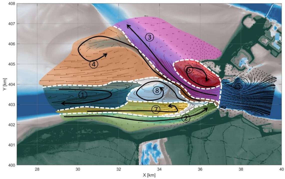
Figure 5.10: 2019 bathymetry with interventions. The dotted white lines indicate boundaries between divergent or non-convergent parallel paths. The black arrows indicate the main sediment pathways.
