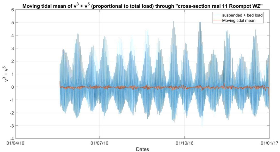
Figure 4.3: An approximation of the suspended + bed load and the moving mean per tidal cycle through the cross section in Figure 4.2.
