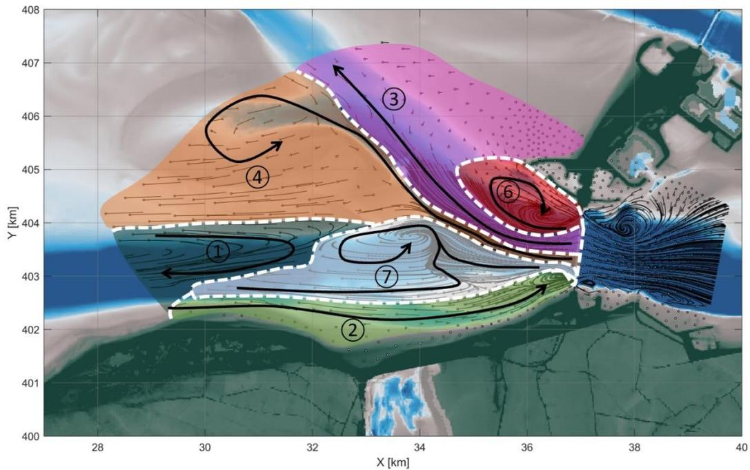
Figure 5.9: 2019 bathymetry with the implemented removal of sediment zoomed in on the Roompot channel. The dotted white lines indicate boundaries between divergent or non-convergent parallel paths. The black arrows indicate the main sediment pathways.
