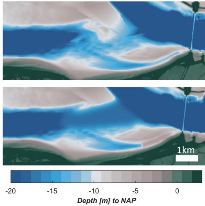
Figure 4.9: Top: 2019 Bathymetry. Bottom: 2019 bathymetry with interventions.
