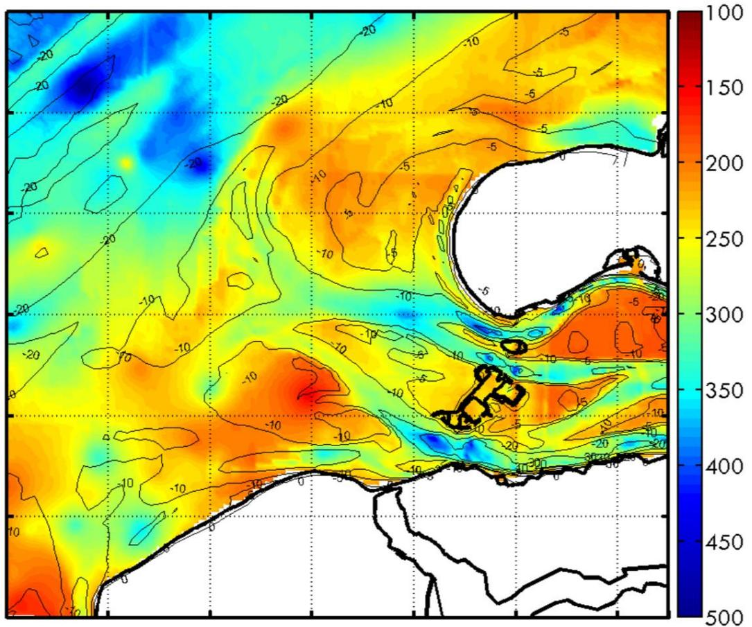
Figure 2.2: Median grainsize ( $d_{50}$ ) on the ebb-tidal delta. The contour lines indicate the depth in m below MSL and correspond to the 2008 bathymetry. Units on the color bar are in microns. (Eelkema, 2013)
