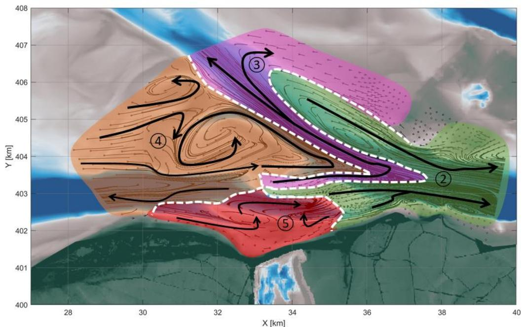
Figure 5.5: 1976 bathymetry without barrier. The dotted white lines indicate boundaries between divergent or non-convergent parallel paths. The black arrows indicate the main sediment pathways.
