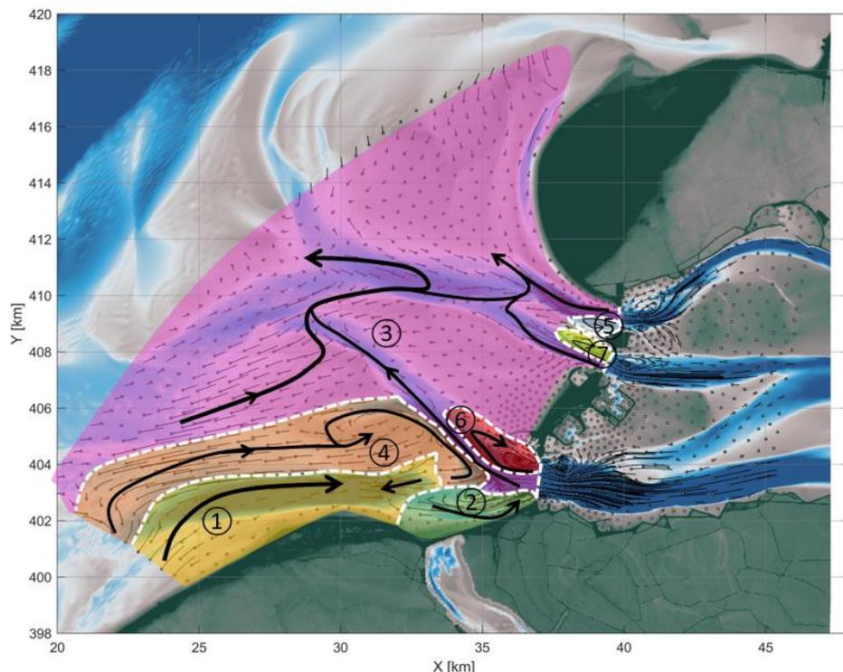
Figure 5.3: 2019 bathymetry with barrier. The dotted white lines indicate boundaries between divergent or non-convergent parallel paths. The black arrows indicate the main sediment pathways.
