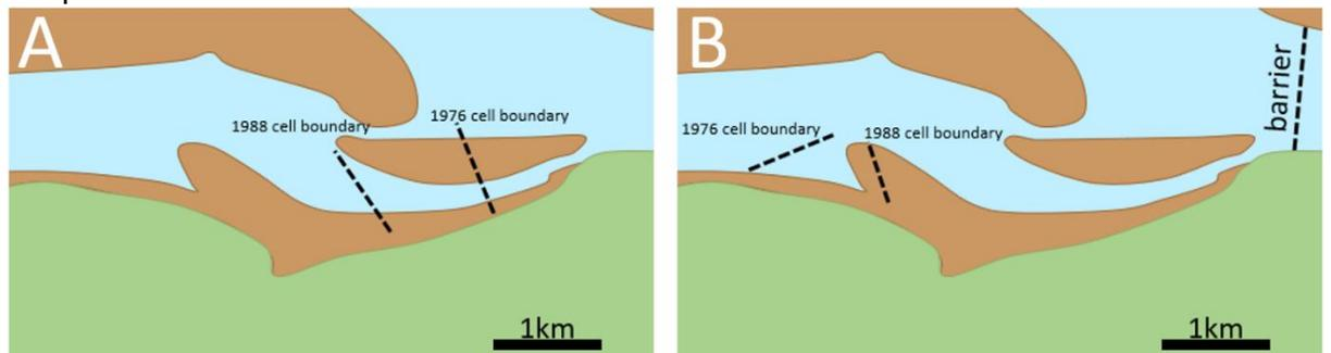
Figure 6.3: Schematization of the sediment sharing cell boundary shift along the coast of Noord-Beveland. A represents the cell boundaries in 1976 and 1988 without the barrier in place. B represents the cell boundaries in 1976 and 1988 with the barrier in place. Both images show the bathymetry of 1988.
