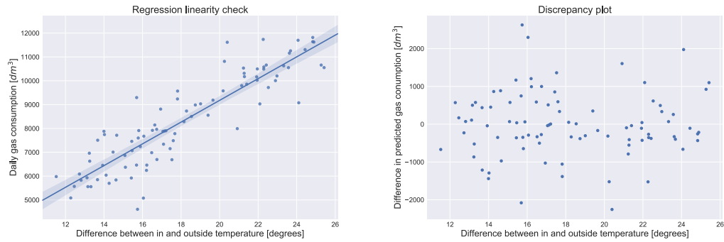
(a) Linearity of gas consumption and inside temperature (b) Difference between the predicted gas consumption and actual gas consumption
