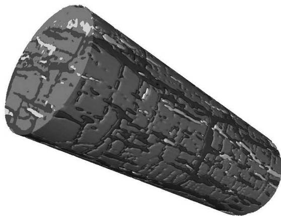
Figure 2.2: Combined view of the CT-scan of the fractures, minerals and matrix of the cylindrical Tupton coal sample.
