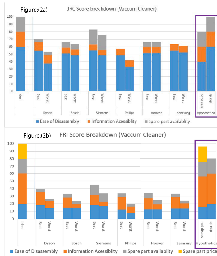
Fig. 2. Score breakdown for vacuum cleaners. 2a = JRC Score, 2b = FRI score, "sp exp" = expensive spare part; "not disass" = a priority part cannot be disassembled.
