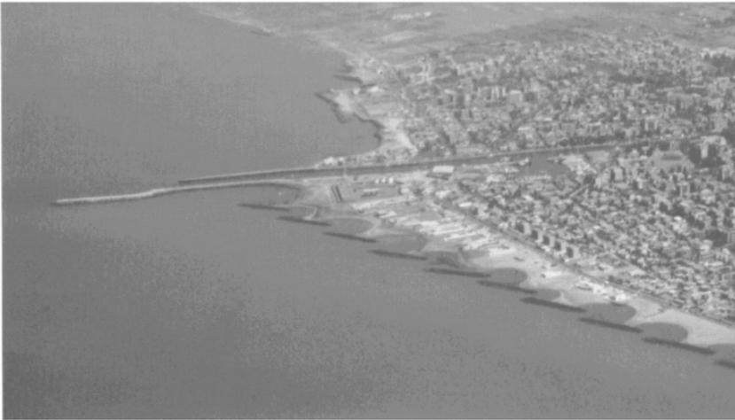
Figure 4-3 A system of detached breakwaters at Fiumicino, Italy.
