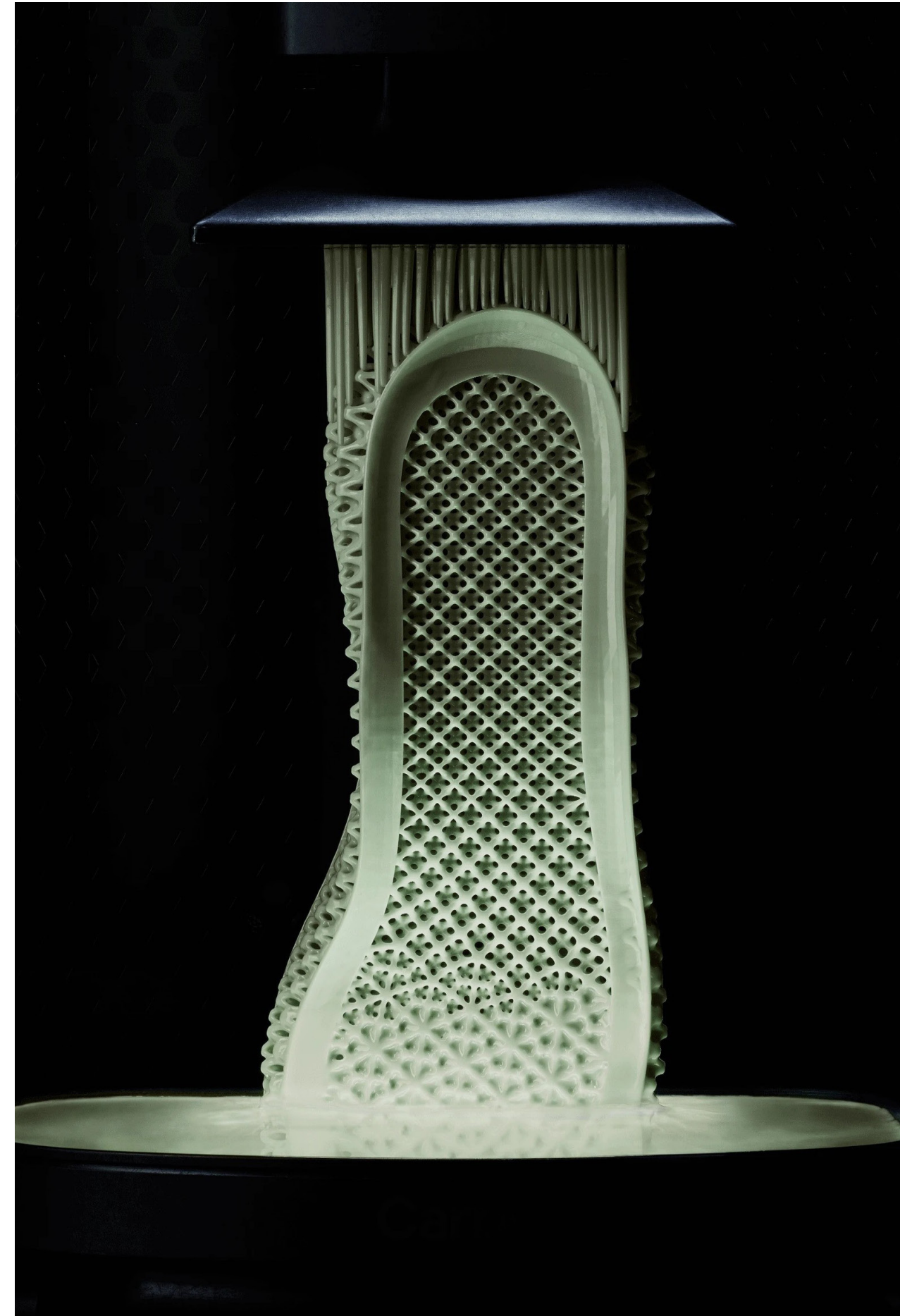
Figure 8: SLA printing process of midsole unit by Carbon and Adidas (Carbon, n.d.)
