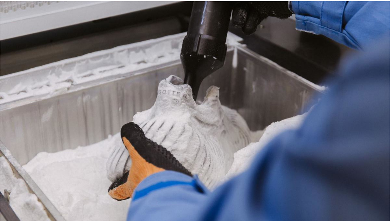
Figure 10: 3D printing process of HP for Botter using Multi Jet Fusion (Ricciardi, 2023)
