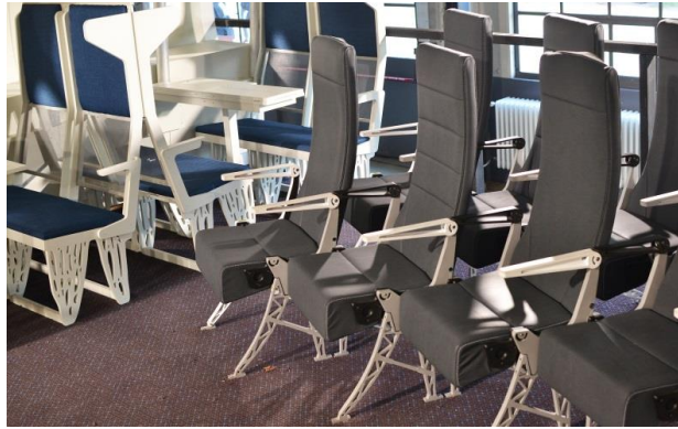
Figure 12: Staggered seats may be added to the cabin of the Flying V to allow passengers more privacy while they sit in the direction of flight. [28]
