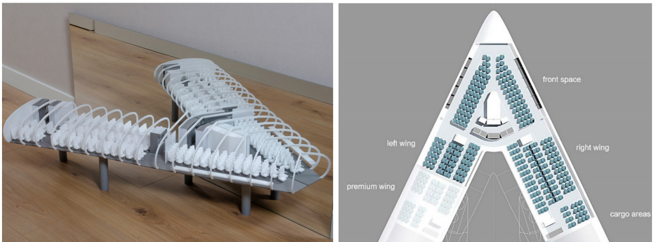
Figure 13: View of an alternative cabin concept for the Flying V. A model is displayed on the left, a schematic view is displayed on the right. [27]
