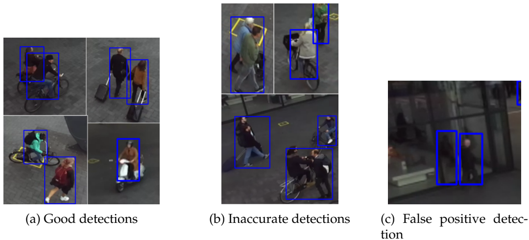
Figure 9.2: Different types of detections based on accuracy for Amsterdam Central data
