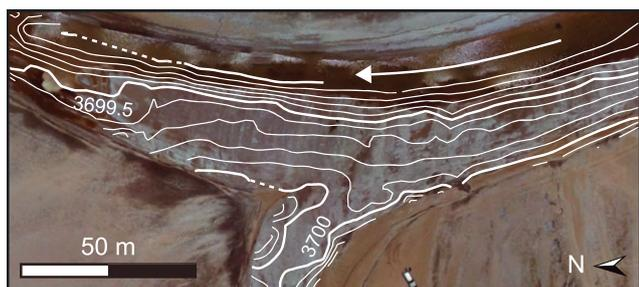
**Figure 8.** KAP orthophoto of an asymmetrical reflux lobe (associated with the crevasse splay in Figure 6A) showing surface topography (white contours). White arrow indicates flow direction in the parent channel. Arrow indicates north. [Colour figure can be viewed at [wileyonlinelibrary.com](http://wileyonlinelibrary.com)]
