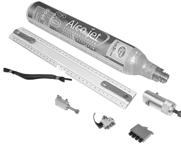
Figure 7.6: The pneumatic components and a 30 cm ruler to indicate their sizes. The components are clockwise arranged according to the \text{CO}_2 flow through the system; 5.8 Mpa \text{CO}_2 canister, the first stage pressure regulator to 1.2 Mpa, a block of four second stage regulators to 0.6 Mpa, one of four low-power SMC TM valves, one of four small SMC TM cylinders and one of four Shadow TM McKibben muscles.
