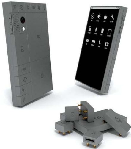
Figure 15 – The modularity of the Phonebloks concept. It increases reusability, but also changes its physical specifications (e.g. the thickness of the phone). Image from www.phonebloks.com
