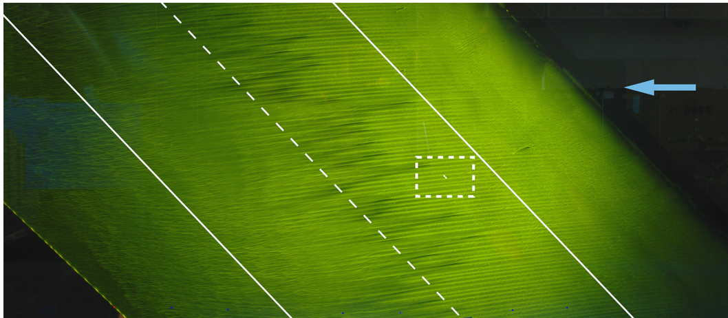
Fig. 3 Fluorescent oil flow visualization on the suction side of the 45° swept wing model installed in the TU Delft LTT wind tunnel at Re = 2.15 \cdot 10^6 and \alpha = -3^\circ . Critical forcing ( \lambda_f = \lambda = 9mm ) case. The white dashed line is the wing mid section x/c = 0.5 , the other two indicate station x/c = 0.25 on the right and station x/c = 0.75 on the left respectively.
