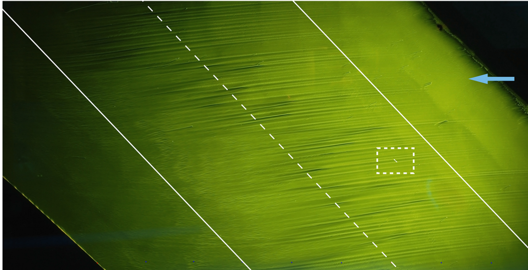
Fig. 6 Fluorescent oil flow visualization on the suction side of the 45° swept wing model installed in the TU Delft LTT wind tunnel at Re = 2.15 \cdot 10^6 and \alpha = -3^\circ . Sub-critical forcing ( \lambda_f = 5mm ) case. The white dashed line is the wing mid section x/c = 0.5 , the other two indicate station x/c = 0.25 on the right and station x/c = 0.75 on the left respectively.
