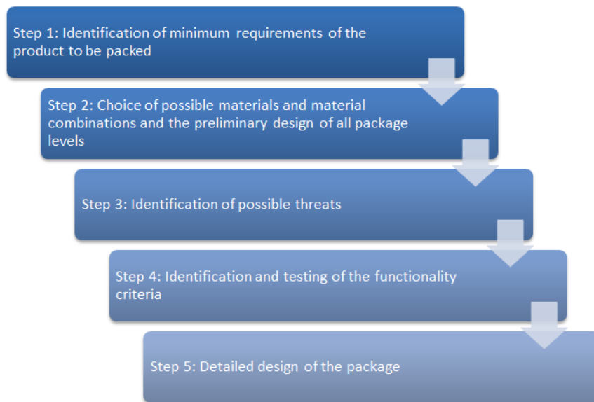
Figure 7: Framework for guiding approach to design sustainable food packaging (Grönman, et al., 2013)
