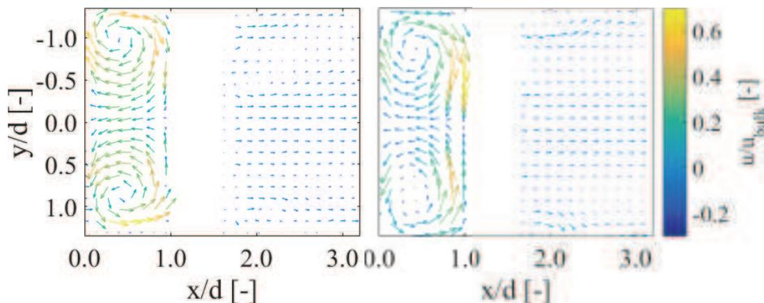
**Fig. 7** Comparison between a steady case and a pulsation case, respectively. The white square is the catalytic dummy. Only every 10 vector in each direction is shown. Both cases are an average of all sampled data.
