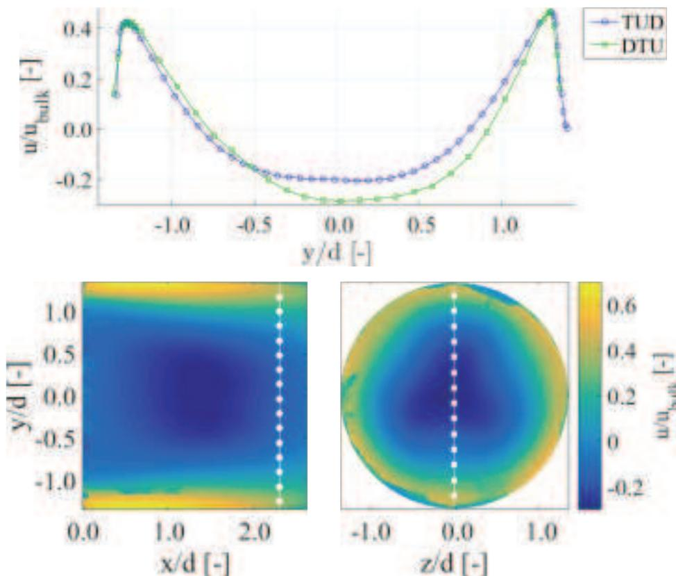
**Fig. 3** Top view shows comparison between the steady cases for the setup at DTU(air) [8] and at TUD(water). Not all points are shown and the full line is used for better visualisation. At the bottom left the TUD case viewing the  $xy$  plane and right the DTU viewing the  $yz$  plane. The two cases overlap at the sample line shown on both plots as white marks.
