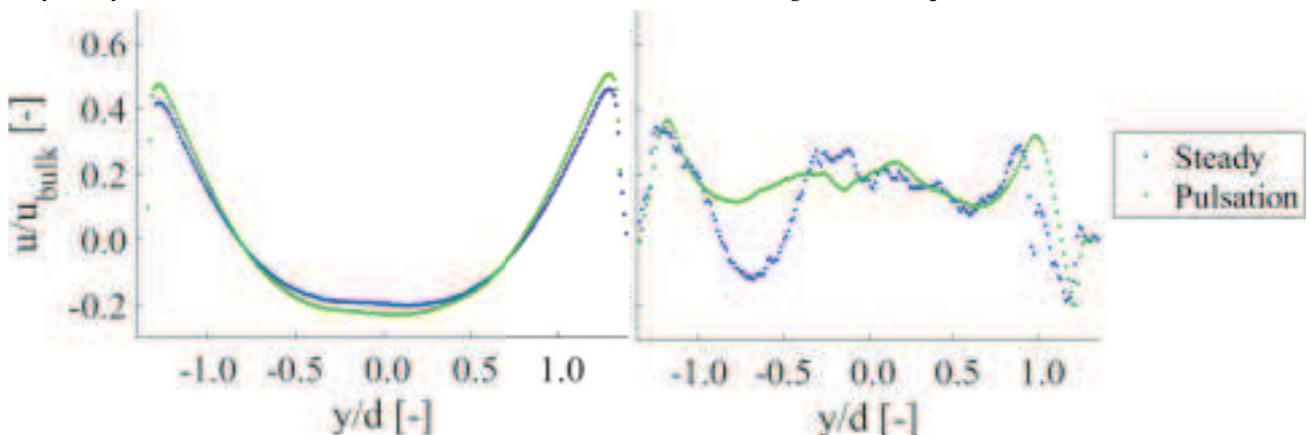
**Fig. 8** Velocity profile comparison at  $x/d = 2$ . Where the left show the cases without catalyst dummy and the right show the cases with a catalyst dummy mounted. Both cases are an average of all sampled data.
