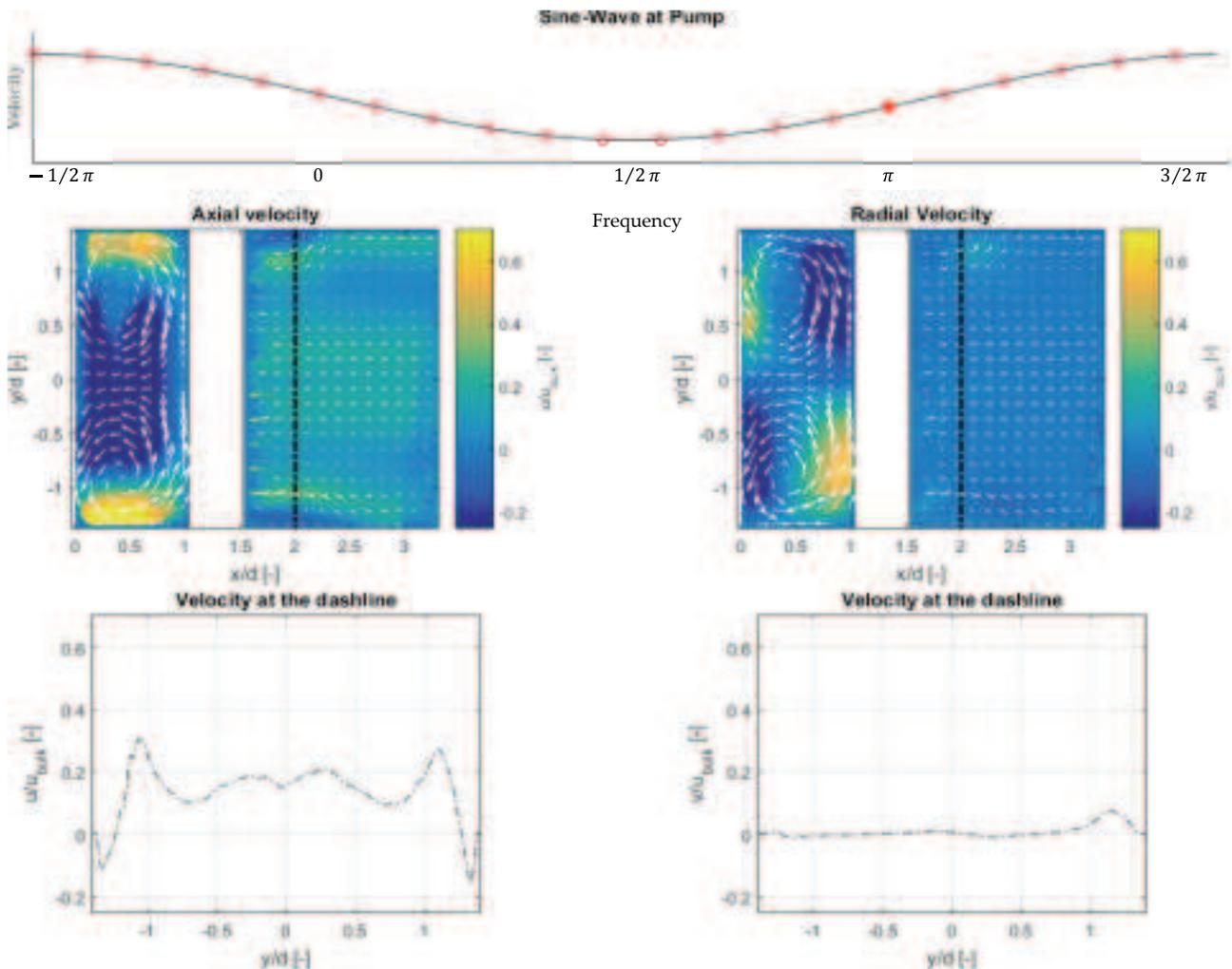
**Fig. 4** Top: The sine wave prescribed to the pump, where the circles indicate the different sampling points and the full dot indicate the present case. Middle: Velocities in the measuring plane, where the white square is the catalyst dummy. The white arrows show the in-plane velocity, the colours show the magnitude of the velocity component, according to the label. Bottom: The velocity profile at the dashed line.
