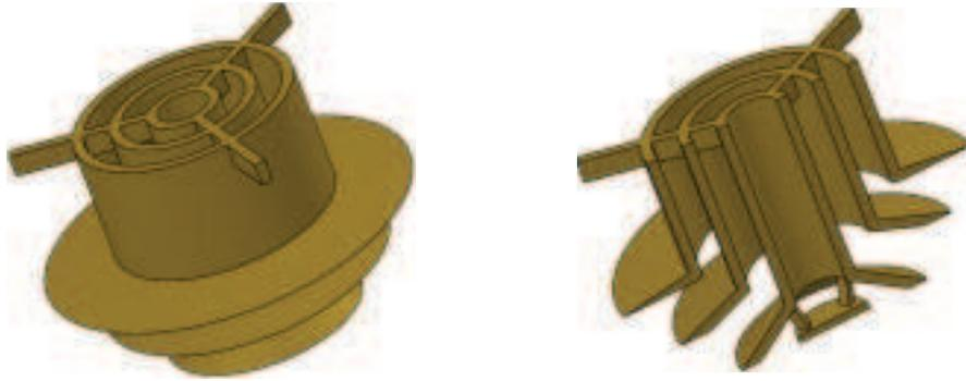
**Fig. 2** Flow distributor/guide vanes, where it is possible to see the tripartite guide vane construction. It is mounted in the sudden expansion.
