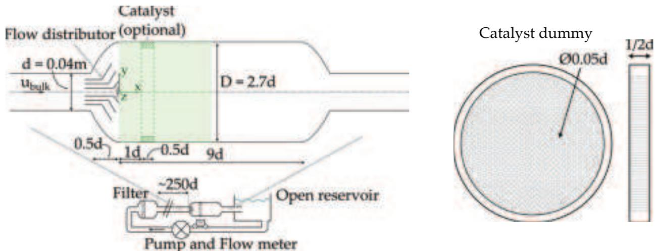
**Fig. 1** Left: Schematic sketch of the setup, where all the important dimensions are shown. The coordinate system is shown on the center axis, just after the expansion. The green area shows the measurement area. Right: A model of the catalyst dummy, with the sizes of the bores shown.
