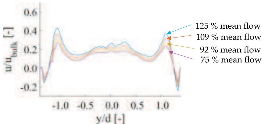
**Fig. 5** Phase average velocity profiles at  $x/d = 2$  with the catalyst dummy mounted. Only data from a half phase is shown going from maximum to minimum. The lines show the velocity at four different amplitudes.
