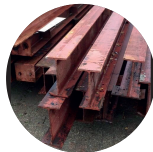
Reclaimed IPE360 (360x- 170x12,7mm) beam from Sint Oedenrode
