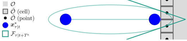
Figure 3.5: Visualization of a scenario in which the robot would crash into the obstacle if the constraints are not tightened. The obstacle is inflated, here represented by \mathcal{O} , with corresponding occupied grid cells \bar{\mathcal{O}} and the point representation of \bar{\mathcal{O}} in the code. While the ellipsoid does not intersect the grid points, it overlaps with the obstacle region, i.e., \mathcal{F} \cap \bar{\mathcal{O}} \neq \emptyset .
