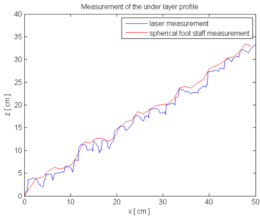
Figure K-6 Measurement from the middle location
