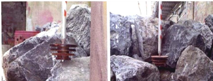
Figure 2-19 Survey with the spherical foot staff. Figure from MEULEPAS et al. , 1999.
