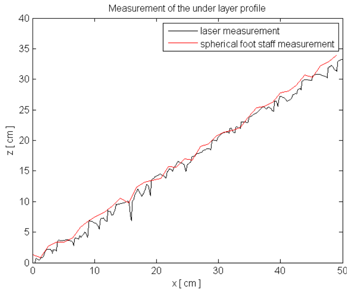
Figure 5-2 Laser and spherical foot staff measurement at the same location
