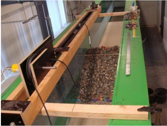
Figure 3-6 Wooden frame with laser device which is used to measure the profile of the under layer
