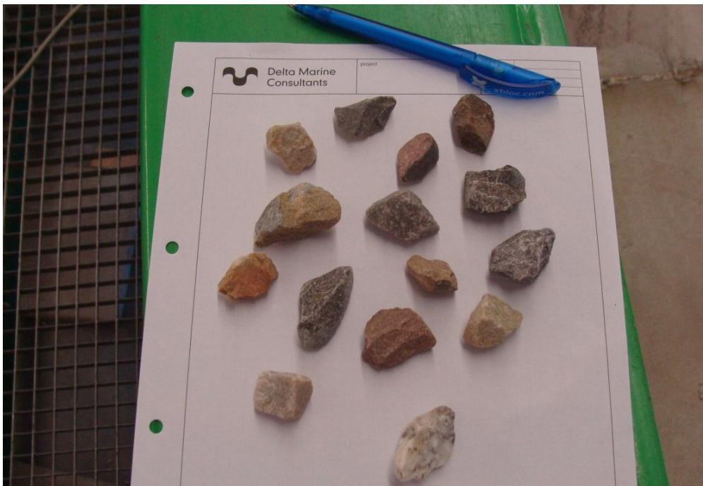
Figure C-2 Stones in the under layer of the model
