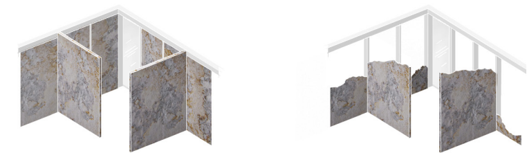
2. PERMANENT STRUCTURE - MYCELIUM INFILL
