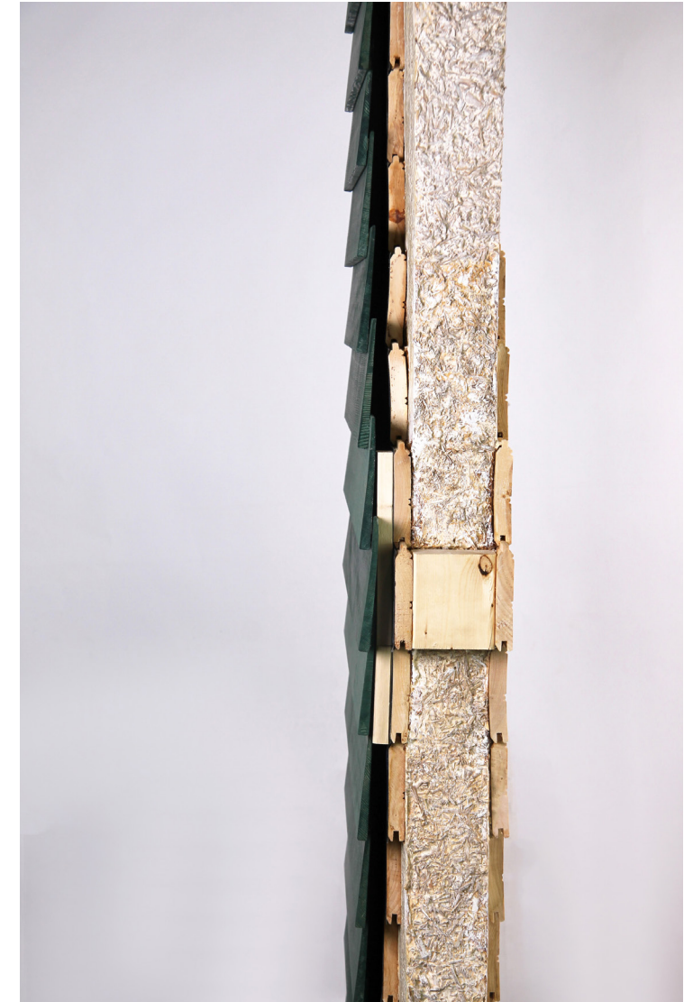
Figure 5: Mycelium insulation material (Ecovative Design, 2007)
