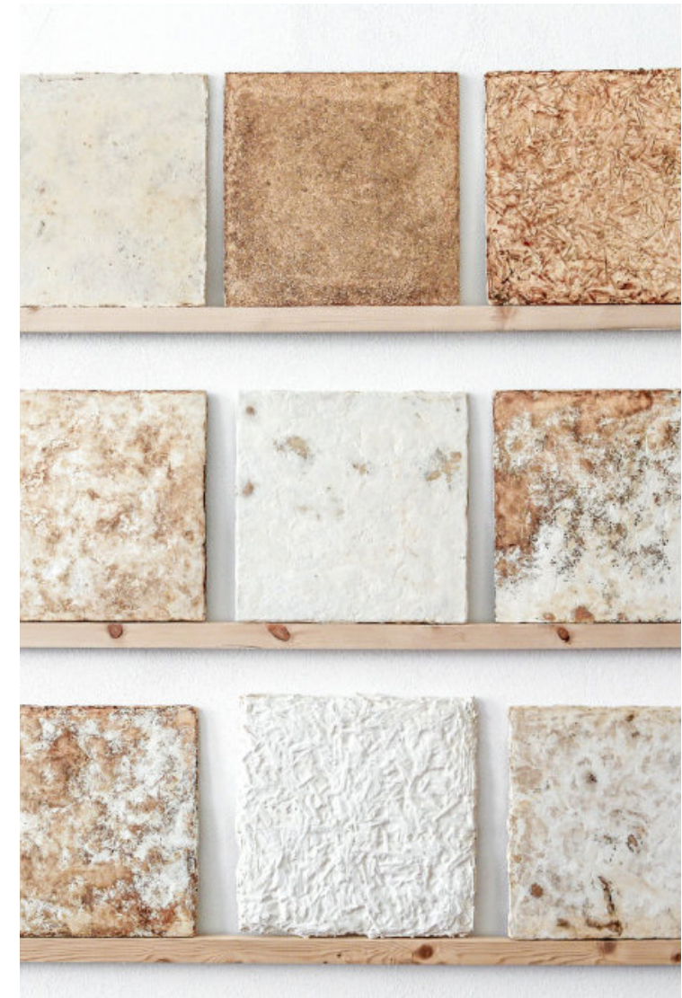
Figure 9: Acoustic panels (Mogu, 2015)
