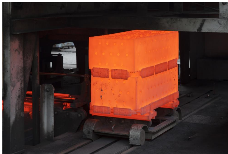
Figure 1.6 A basket of heat-treated GJMW just coming out the furnace. Source: Nefit Industrial
