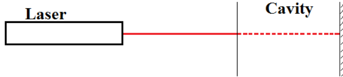
Figure 2.5: A schematic setup of an optical cavity.
