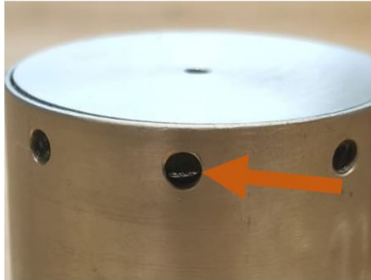
(a) The "bulged-out" o-ring
