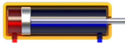
Figure 4.1: A double acting pneumatic cylinder. Image taken from [21]
