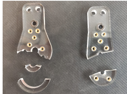
(b) The broken PMMA sheets
