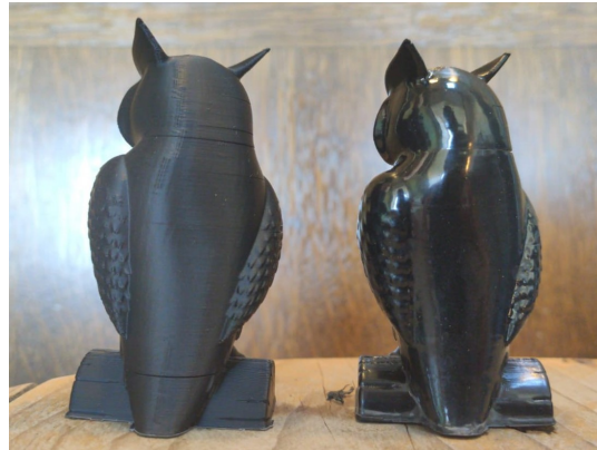
Figure 5.10: The effects of an acetone treatment on ABS. On the left: Untreated, on the right: Treated with acetone
