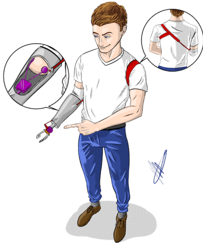
Figure 1: Visualization of body powered and externally powered control. Body powered prostheses utilize movements of other bodyparts, e.g. by means of a harness and a cable to harness the movements of the shoulder (in red), to control and power the prosthesis. Externally powered prostheses use the muscle activity of unused muscles in the stump as signal inputs to control the prosthesis. These signals are picked up by myoelectric sensors (in purple). These prostheses obtain their actuation from an external energy source, e.g. battery or pressurized gas in a cylinder.
