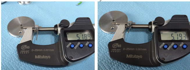
(c) One groove is measured with the auxiliary shafts in the grooves on both sides. (d) The other groove is measured in a similar manner.
