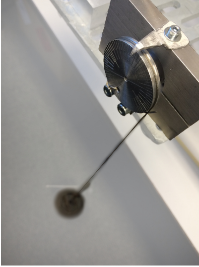
Fig. 11: A cable goes around the wheel to ensure a constant moment arm. by applying different masses the torque on the axle changes.
