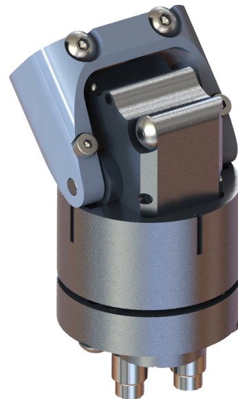
Fig. B.1: Shown is a 3D render of the full design of the wrist mechanism with two vane cylinders (actuators), and therefore two degrees of freedom. The rotation movement is accounted for in the lower part of the design. Where flexion is in the top part. The grey part is in a flexed position of the top vane cylinder.
