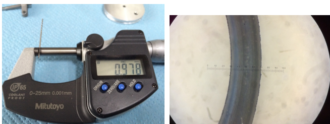
(a) Measurement of two shafts. Both had the same measurement. (b) O-rings are measured under a microscope. With a scaling factor of 40:1.
