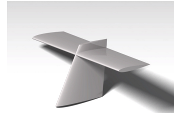
Figure 10.39: T-Tail - Crucifix Hybrid
