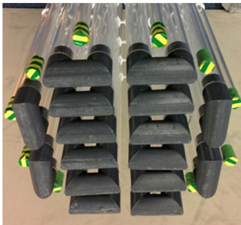
Fig. 2. Picture of “U-connectors” (configuration: internals arranged in squares).
