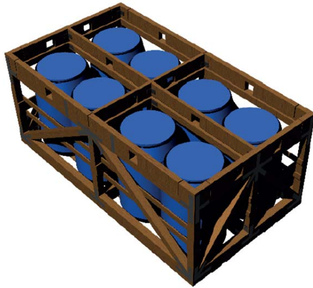
Figure 10.5: timber cage with barrels
