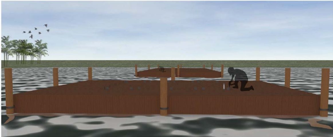
Figure 10.24: coupled foundation modules
