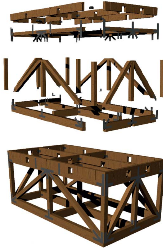
Figure 10.3: creating a timber cage with steel connections
