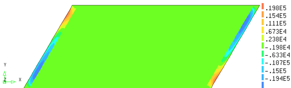
Figure 50, transversal moments with the presence of end beams [Nmm/mm]
