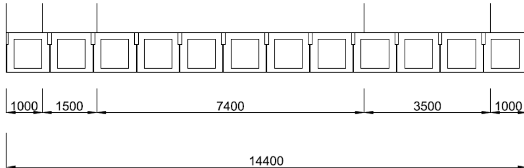
Figure 10, cross-section viaduct – dimensions in [mm] (12 box girders)
