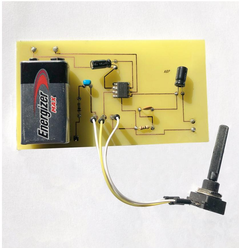
Figure A.6: Final PCB for acoustic stimulation
