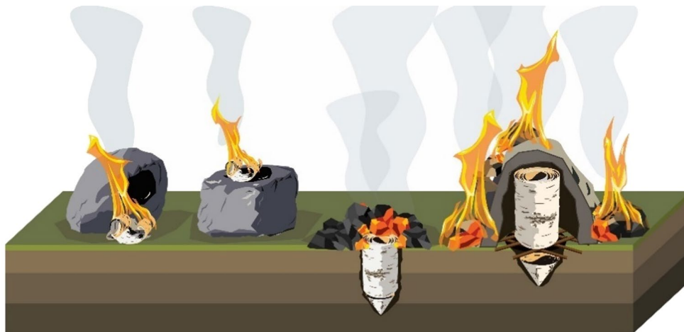
Fig. 1 Different birch tar production methods. From left: vertical condensation, horizontal condensation, pit roll, raised structure
