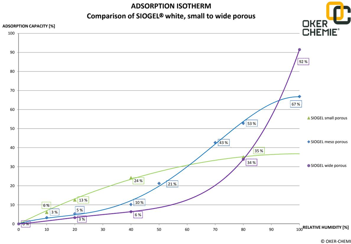
Figure 3.5: Comparison of macroporous, mesoporous and microporous SIOGEL, retrieved from Oker-Chemie GmbH.
