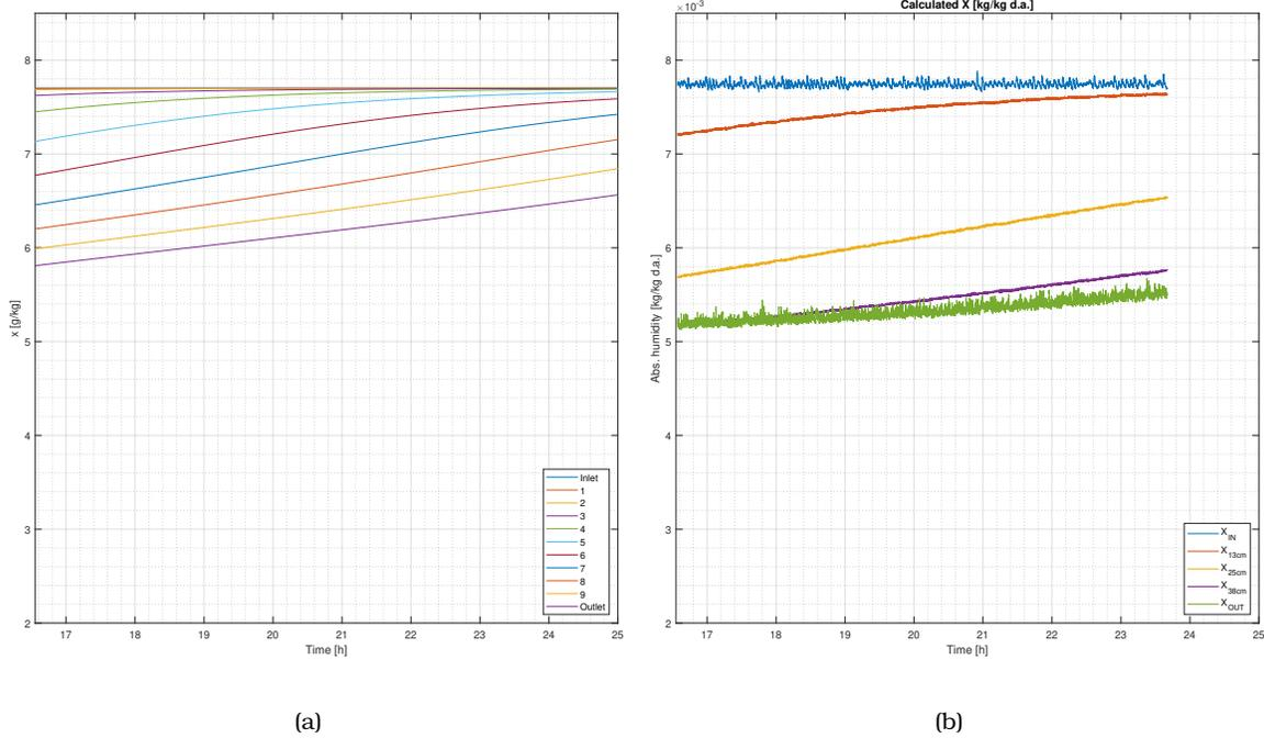
Figure 5.8: Step input from 20 to 50 %RH: (a) PGC model results and (b) experimental results.
