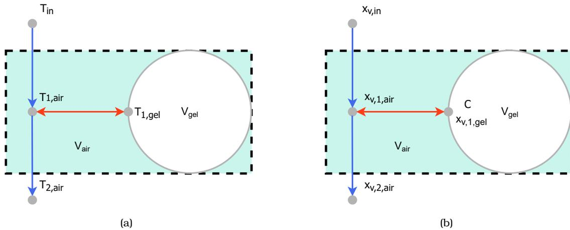
Figure 5.2: (a) Heat flows and (b) mass flows between nodes of finite volume.
