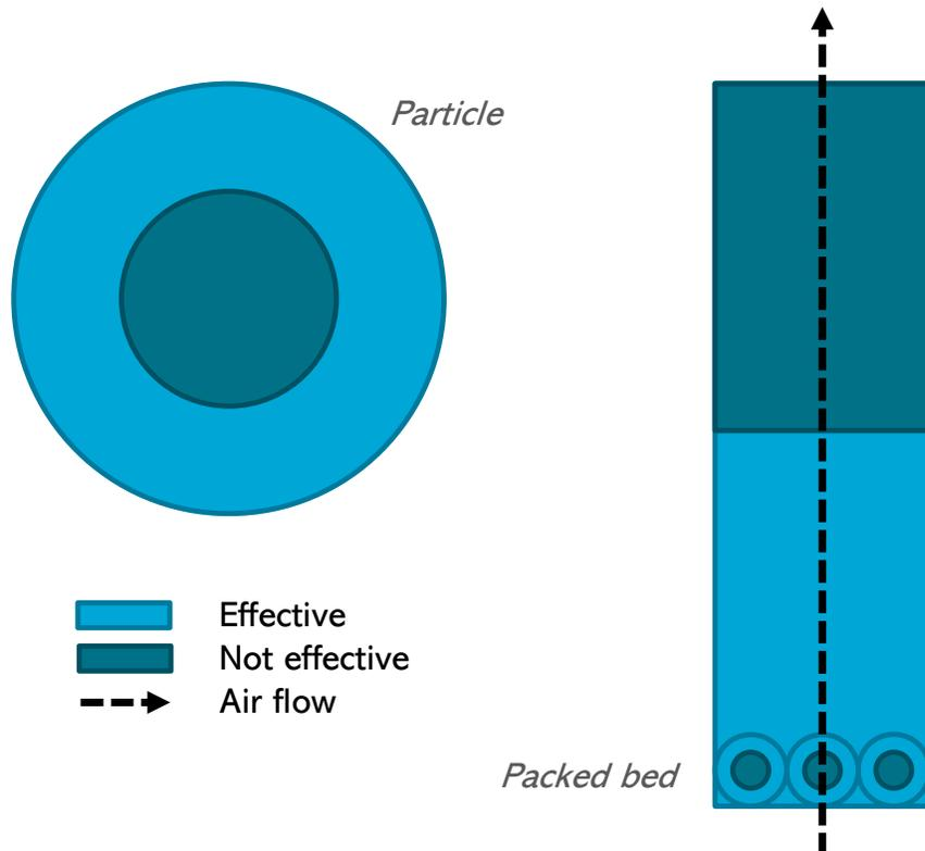
Figure 7.1: Effective volume of silica addressed for a specified humidity fluctuation.
