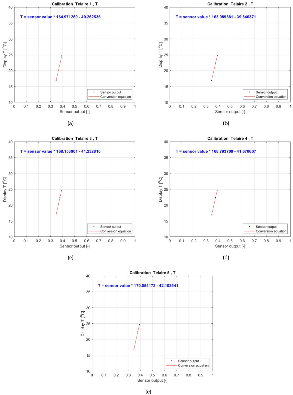
Figure D.3: Temperature calibration of Telaire 1 to 5.
