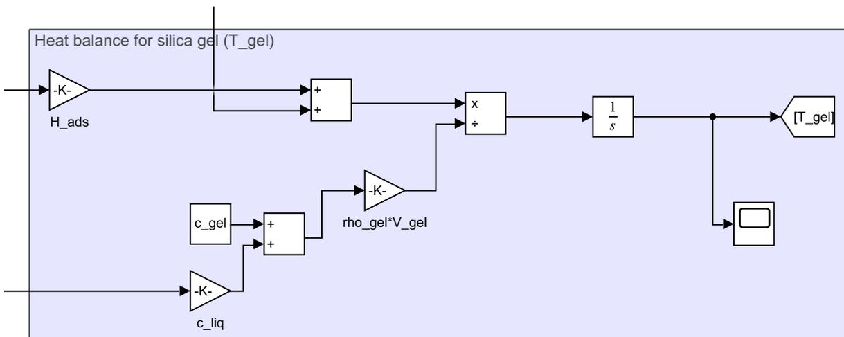
Figure H.5: Heat balance for silica gel.
