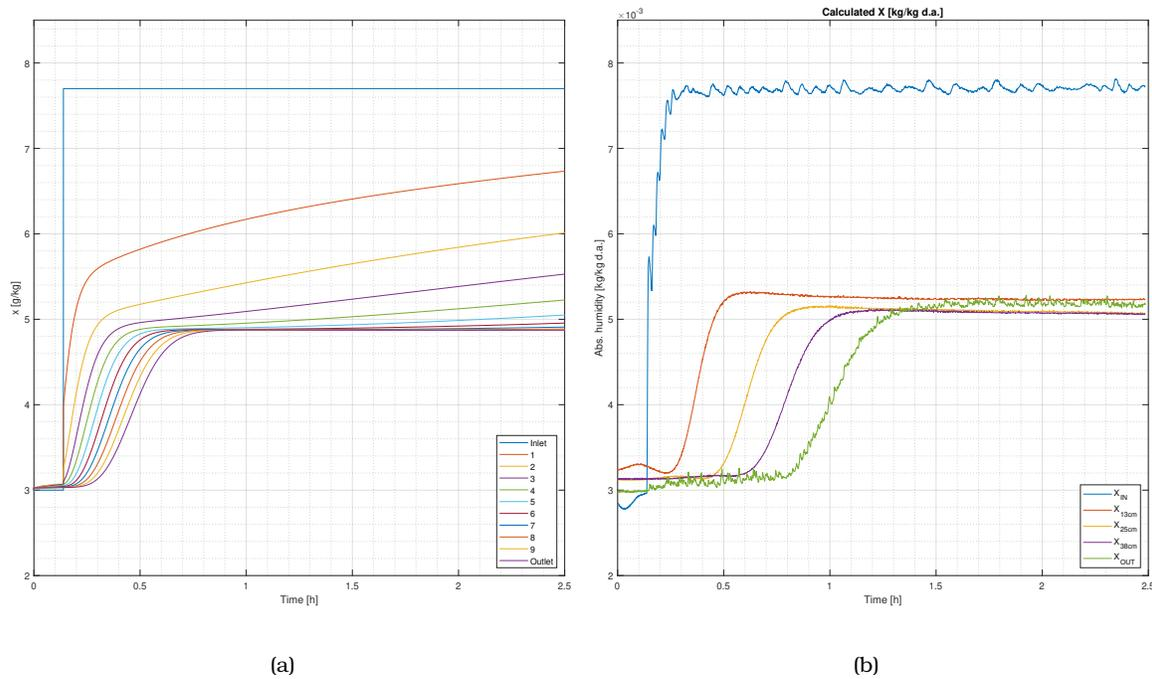
Figure 5.7: Step input from 20 to 50 %RH: (a) PGC model results and (b) experimental results.
