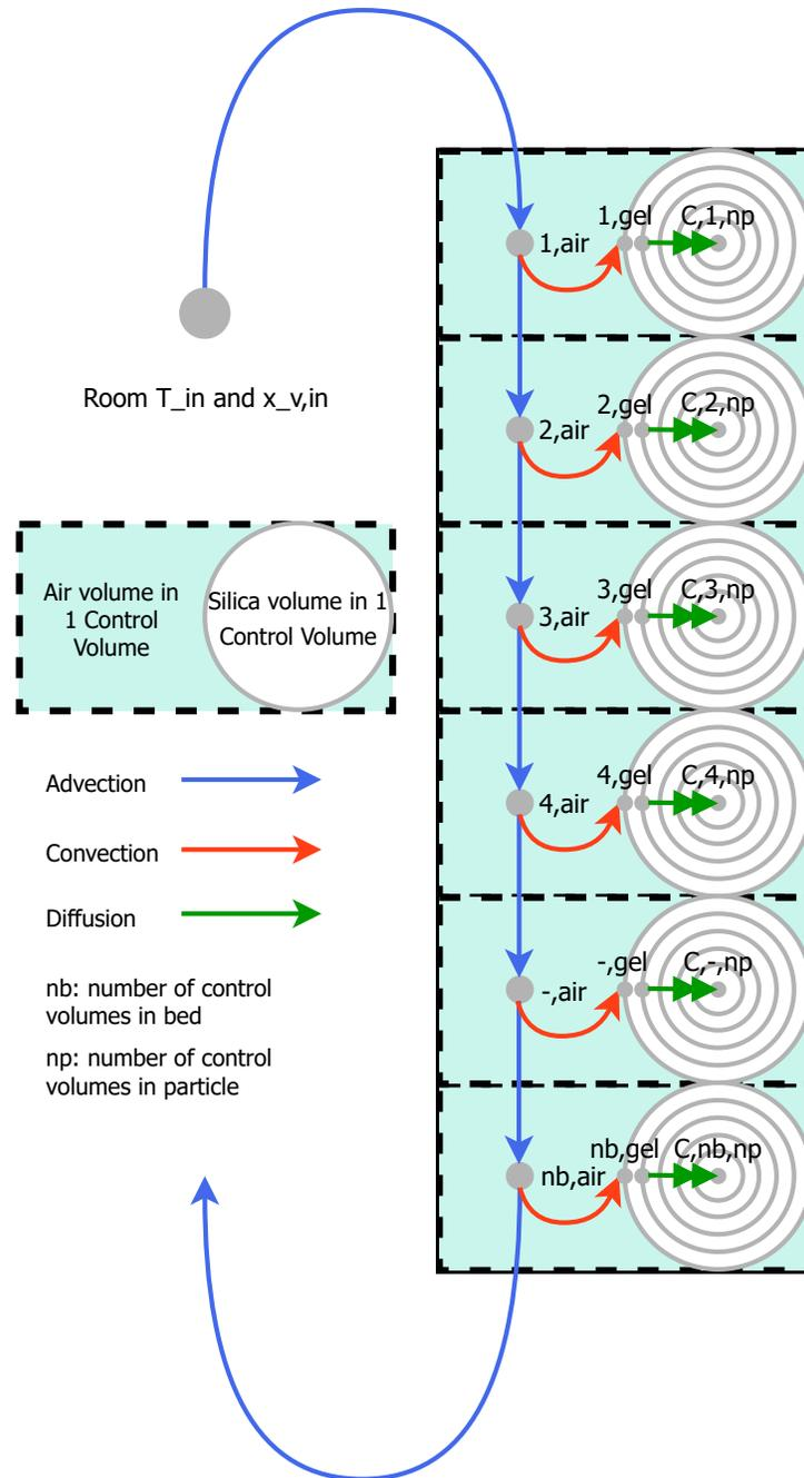
Figure I.2: Schematic overview of the Solid-Side-Resistance model.
