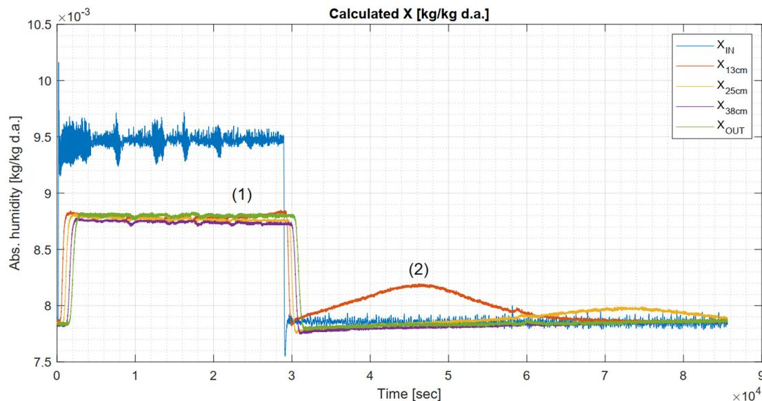
Figure 4.12: Absolute humidity measurements in run 5, cycle **1**.
