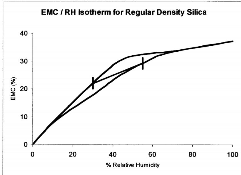
Figure 2.3: Hysteresis and determination of corrected buffering capacity, obtained from [25].
