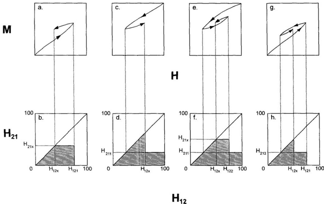
Figure 2.8: Consecutive: (a) Ads - Des, (b) Des - Ads, (c) Des - Ads - Des, (d) Ads - Des - Ads, and corresponding states of both domains, obtained from [1].
