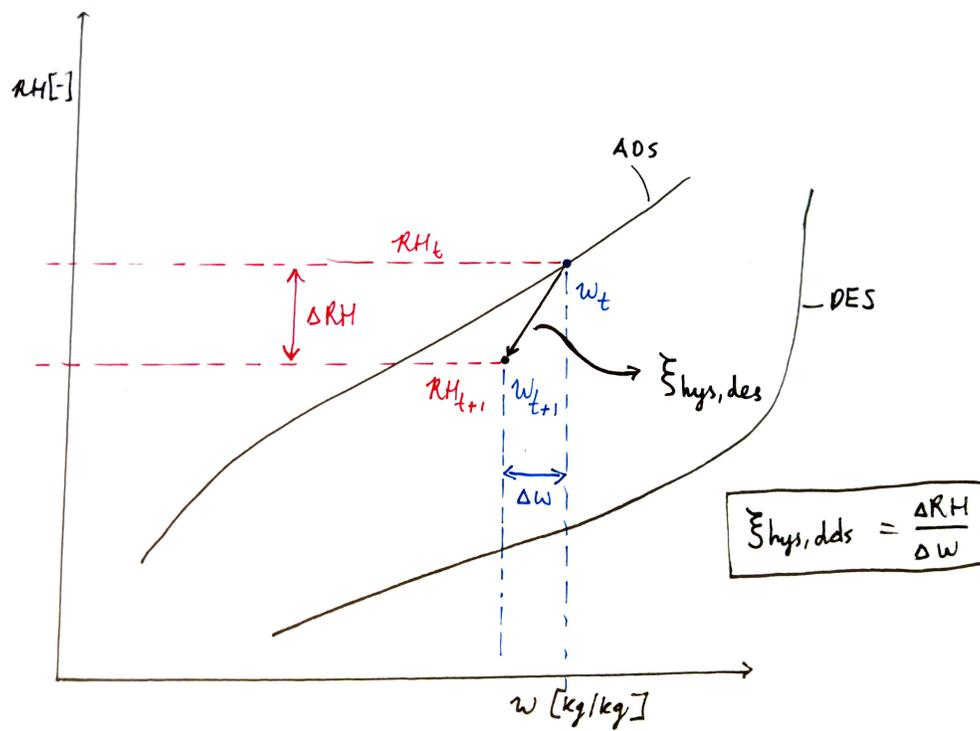
Figure J.2: Calculation of  $RH_{t+1}$ , presented for the case of desorption following adsorption.
