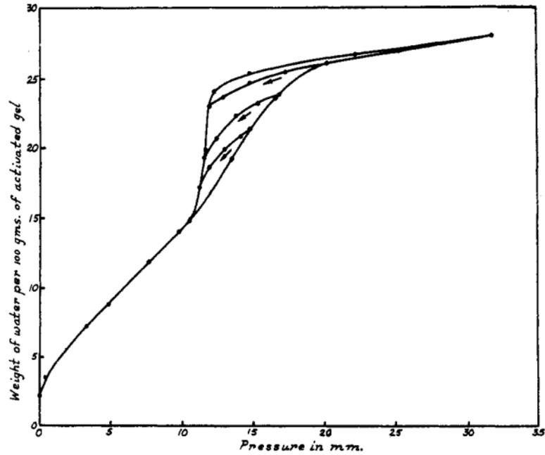
FIG. 2. Scanning of the hysteresis loop in the sorption of water on silica gel
