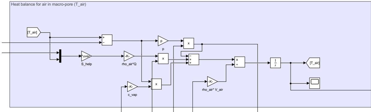
Figure H.6: Heat balance for air in packed bed.
