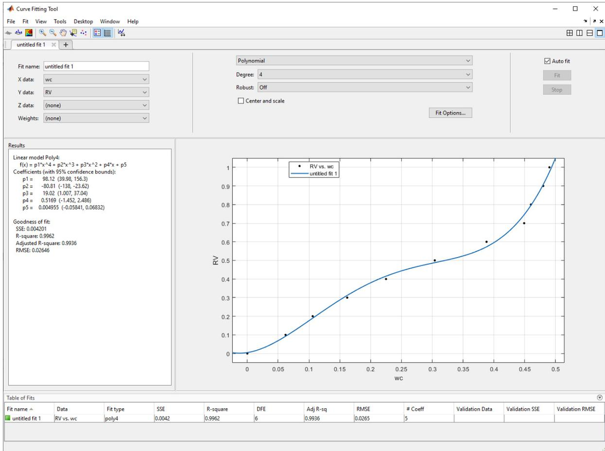
Figure 5.3: Polynomial fitting of  $RH(w)$  using *cftool* in Matlab, with (offsetted) data from uptake rate measurements for sample 6.
