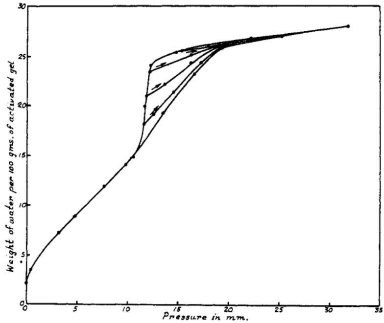
FIG. 3. Scanning of the hysteresis loop in the sorption of water on silica gel
