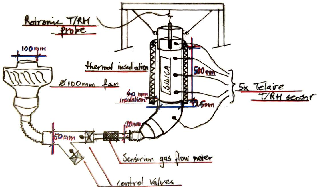
Figure 4.3: Sketch of experimental setup built for Experiment 2.
