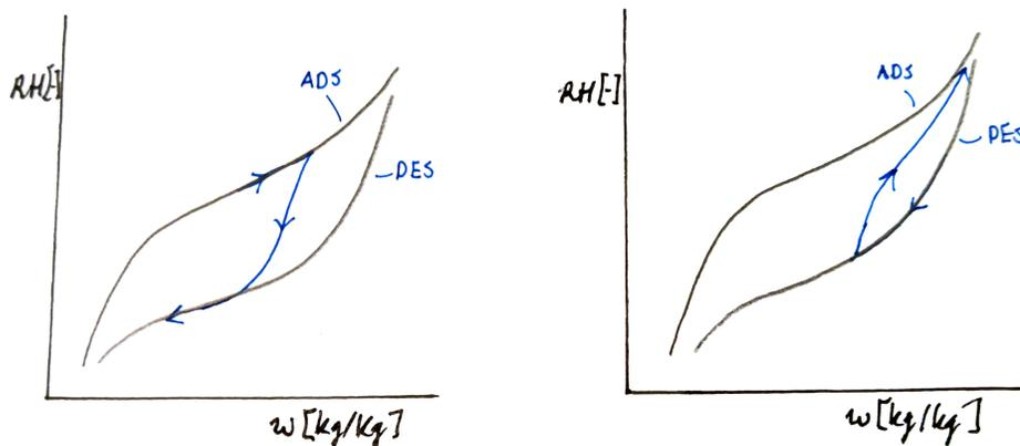
Figure J.1: Scanning curves shown in a  $RH(w)$  plot, for desorption following adsorption (left) and adsorption following desorption (right).
