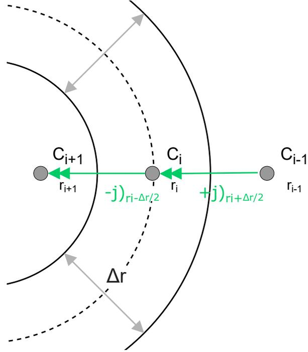
Figure I.1: Mass balance of particle control volume.
