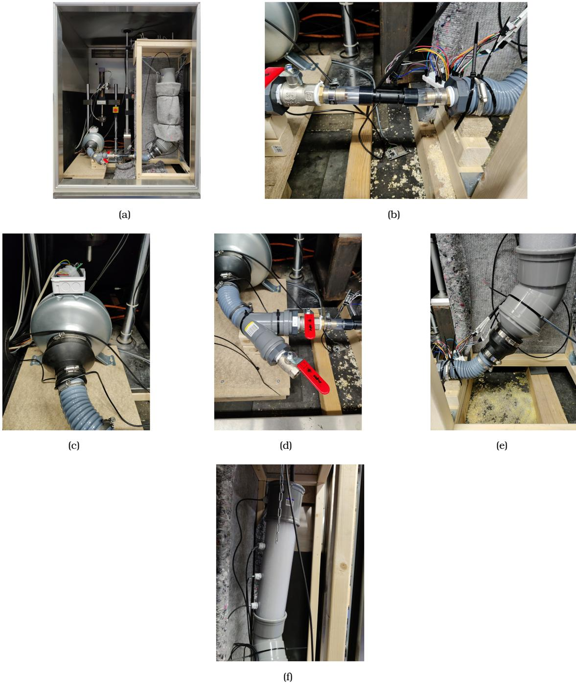
Figure 4.4: (a) Complete setup (b) air flow sensor (c) fan (d) Y piece to regulate air flow (e) packed bed inlet (f) filled packed bed and cable glands.
