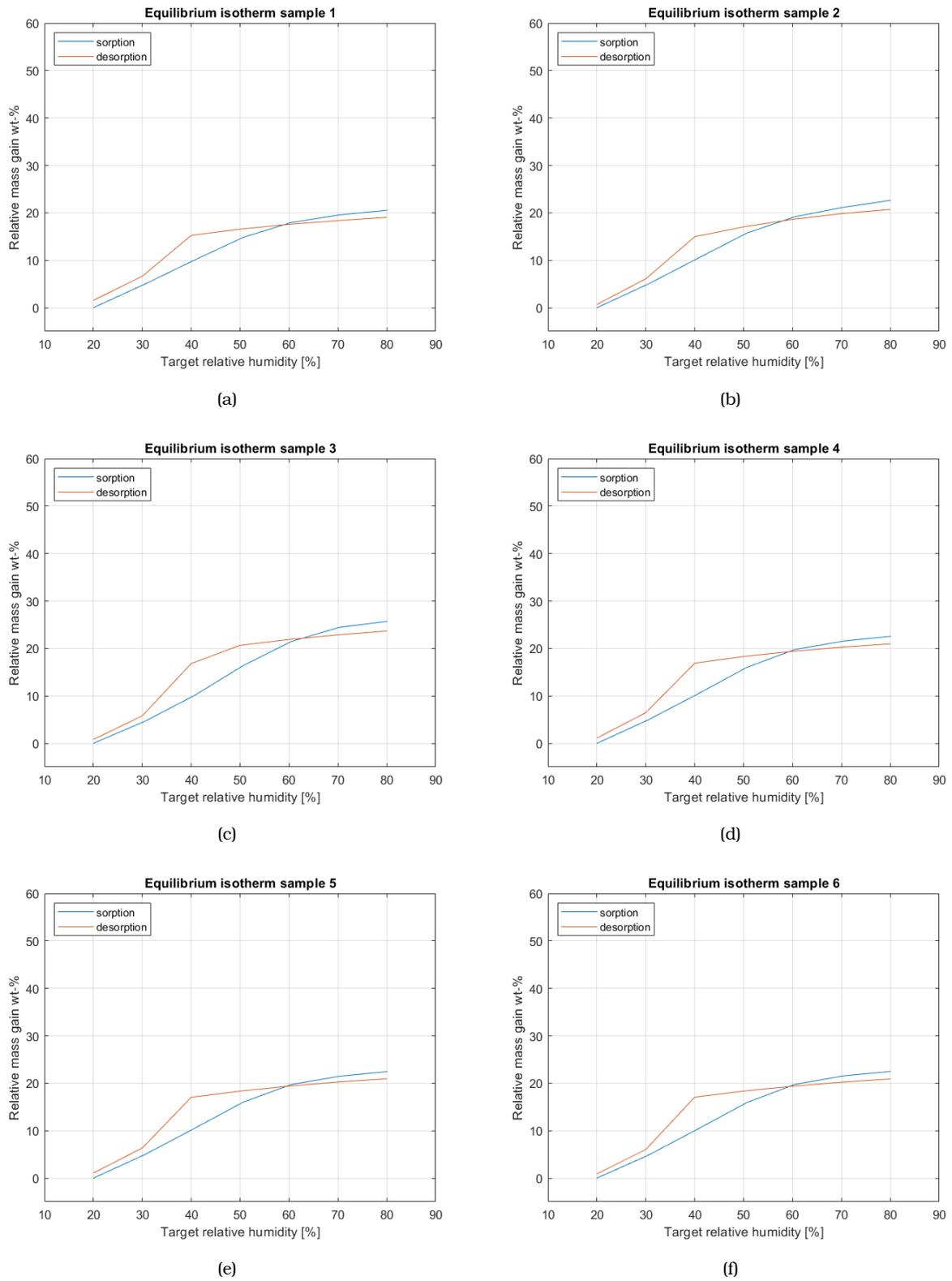
Figure 3.4: Isotherms of samples 1 to 14.
