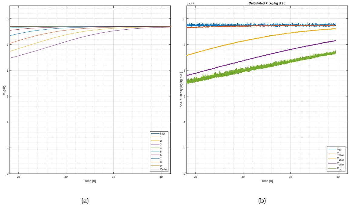
Figure 5.9: Step input from 20 to 50 %RH: (a) PGC model results and (b) experimental results.
