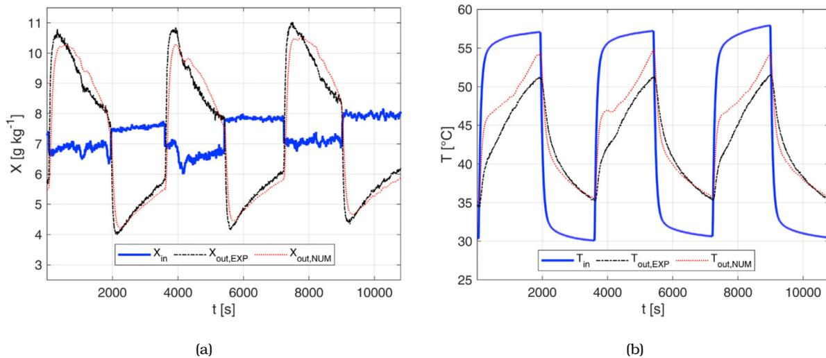
Figure 2.6: PGC-model results by [8] for: (a) response of outlet air humidity to changing inlet air absolute humidity and (b) response of outlet air temperature to changing inlet air temperature.
