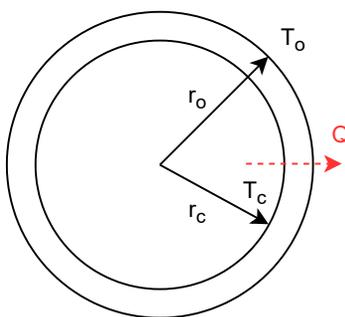
Figure 4.14: Calculation of radial heat conduction (insulation of pipe)
