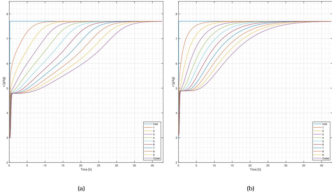
Figure 5.4: Numerical results for a step input from 20 to 50 %RH, obtained with (a) PGC model and (b) simplified model.
