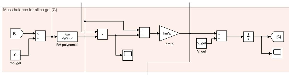
Figure H.3: Mass balance for silica gel.
