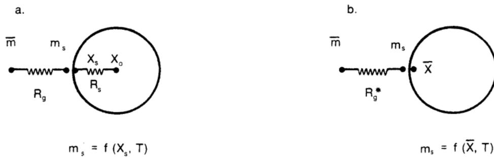
Figure 2.2: (a) Solid-side resistance (SSR) model (b) Pseudo gas-controlled (PGC) model, obtained from [2].
