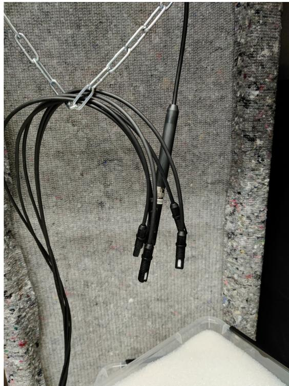
Figure D.5: T/RH sensors hanged together in climatic cabinet for calibration
