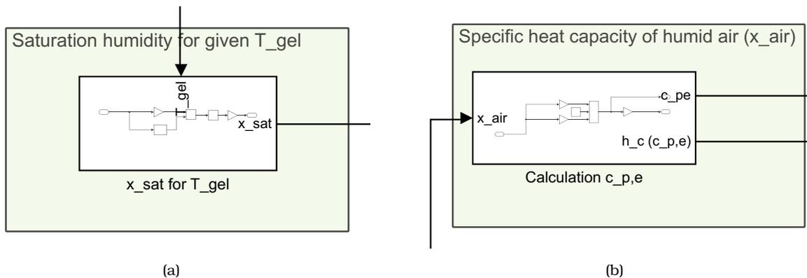
Figure H.7: Calculation of coupling coefficients (a) saturation humidity  $x_{sat}$  and (b) specific heat of humid air.
