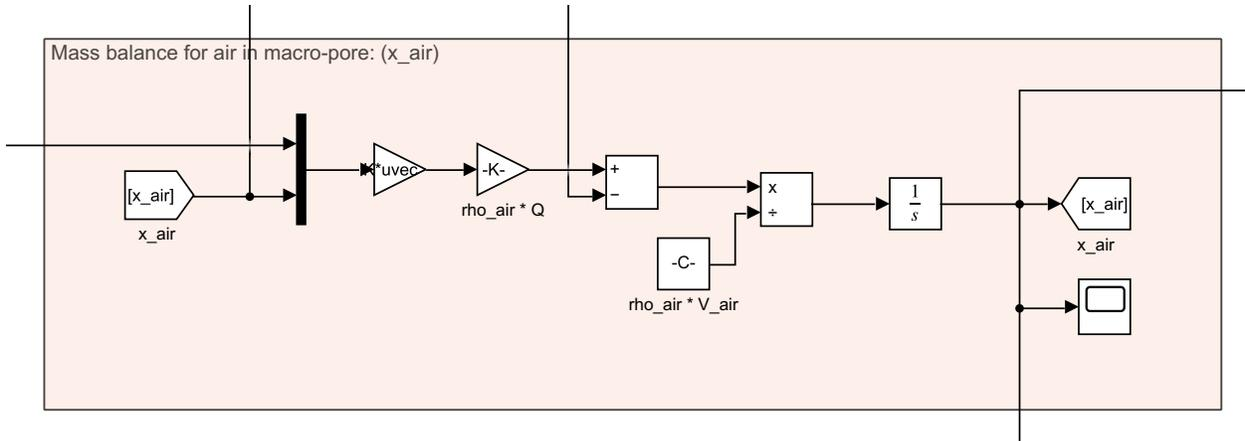
Figure H.4: Mass balance for air in packed bed.
