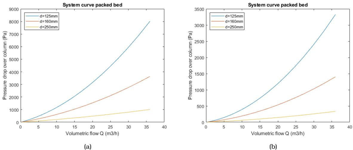
Figure 4.1: Pressure drop over packed bed of  $L = 50$  cm and particle radius (a)  $R_p = 0.001$  m, (b)  $R_p = 0.002$  m
