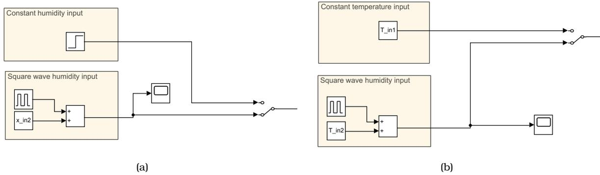
Figure H.2: Model input: (a) inlet air humidity and (b) inlet air temperature.
