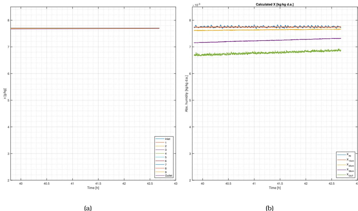
Figure 5.10: Step input from 20 to 50 %RH: (a) PGC model results and (b) experimental results.
