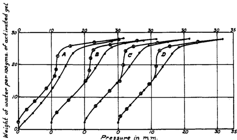
FIG. 1. Hysteresis loop in the sorption of water by silica gel. A, first sorption (●) and desorption (○); B, second sorption (●) and desorption (○); C, third sorption (●) and desorption (○); D, nineteenth sorption (●) and desorption (○).
