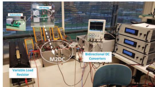
Figure 5: M2DC Experimental Prototype Setup.
