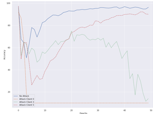
Figure 3: Effects of the veiled MinMax attack on a network from different malicious clients on a ResNet network for the Cifar-10 task. The malicious client in an overlapped region is able to be very effective, while those within a reach of a single server can barely affect the accuracy.
