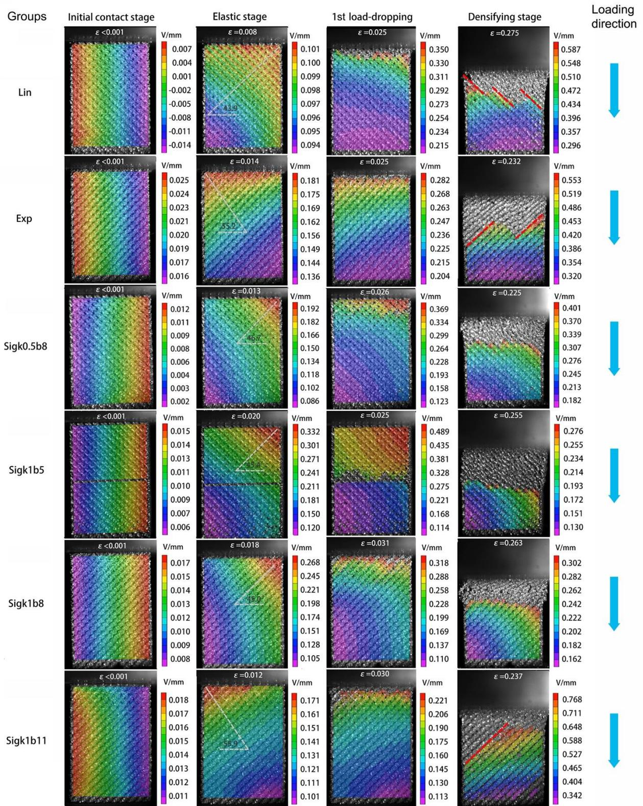
Fig. 15 Vertical displacement ( $d_v$ ) contour at the four stages of the stress-strain curve of every specimen during compression testing: initial contact stage, elastic stage, 1th load dropping stage and densification stage (from left to
