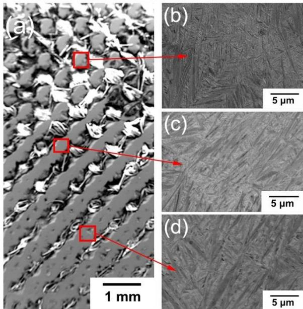
Fig. 3 (a) SEM image of a graded porous structure with a sigmoid function and the microstructures of the areas with porosities of (b) 70%, (c) 55% and (d) 41%.
