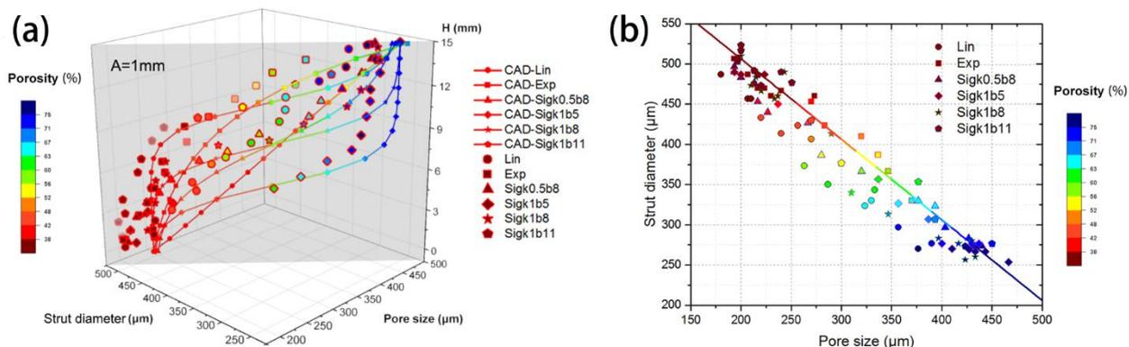
Fig. 9 (a) Variations of strut diameter and pore size with sample height ( $H$ ), in which porosity is expressed by contour legend, and (b) a projection of the data points in (a) on a selected strut diameter-pore size plane.
