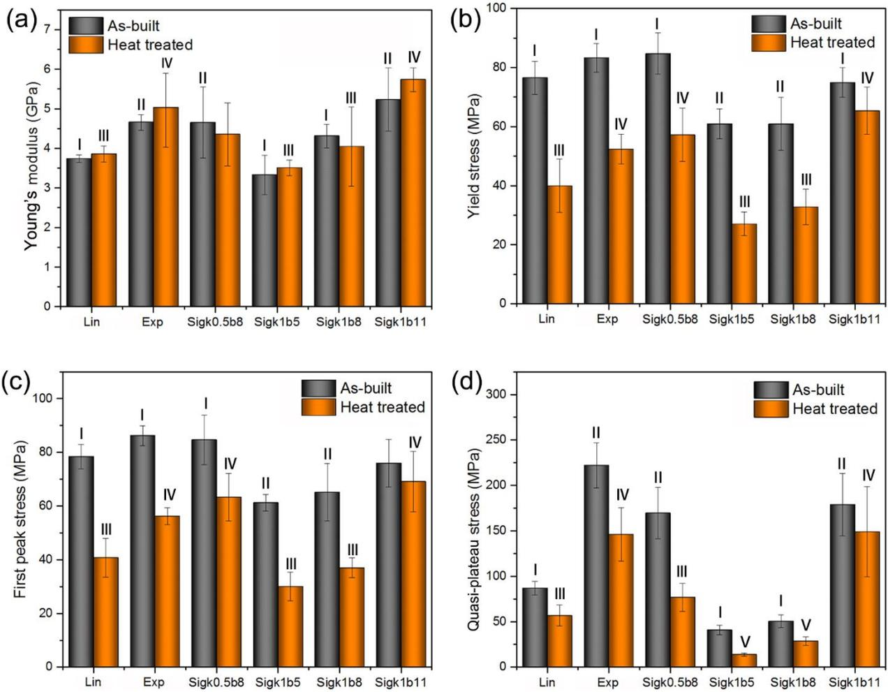
Fig. 13 Mechanical properties of the FGSs: (a) Young's modulus, (b) yield strength, (c) first peak stress and (d) quasi-plateau stress. The test groups marked with the same letter (I, II, III, IV and V) are not significantly different ( $p > 0.05$ ) (one-way ANOVA, Tukey's test).
