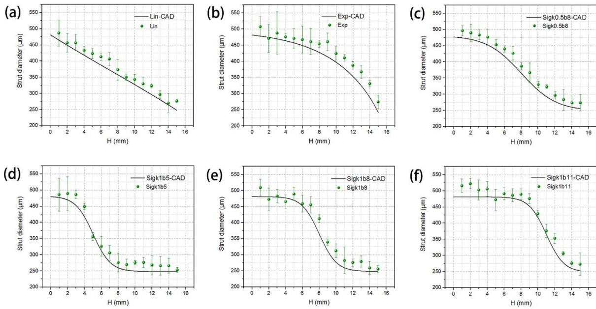
Fig. 7 Comparison in the variation of strut diameter with sample height between CAD design and the as-built samples: (a) Lin, (b) Exp, (c) Sigk0.5b8, (d) Sigk1b5, (e) Sigk1b8 and (f) Sigk1b11.
