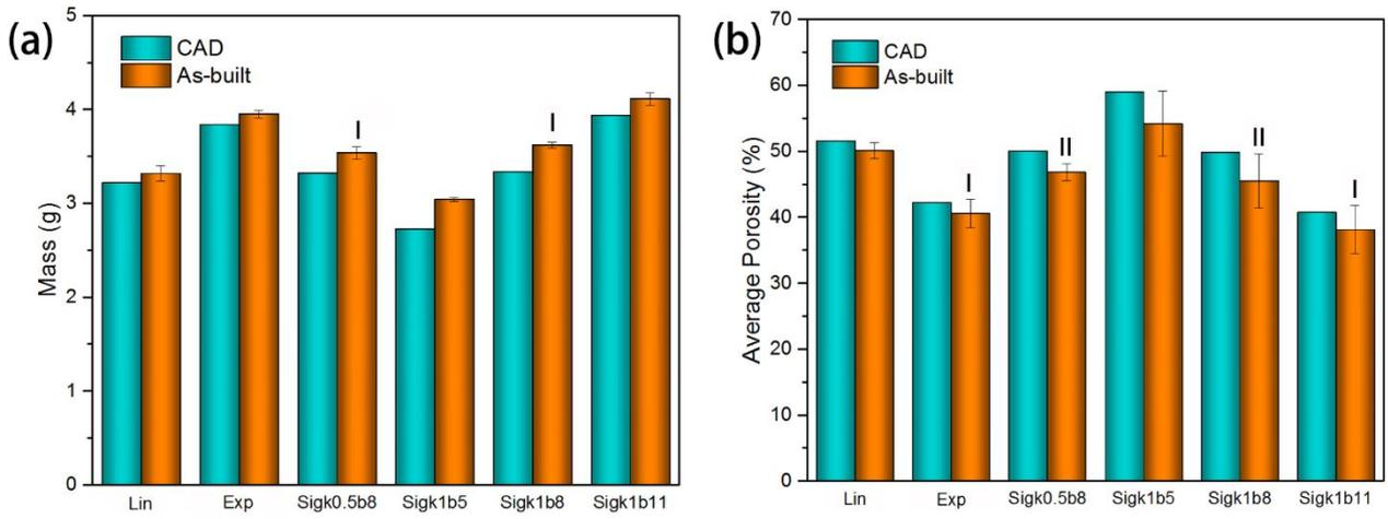
Fig. 5 Comparison between CAD designs and the as-built samples in: (a) mass and (b) average porosity. The test groups marked with the same letter ( I or II) are not significantly different ( $p>0.05$ ) (one-way ANOVA, Tukey's test).
