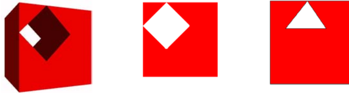
Fig 6 Left: Invalid polyhedron, because the hole divides the polyhedron in two volumes. Note that this object is stored as one volume minus a hole (2 connected inner rings) and not as two separate volumes. Centre: Invalid polygon (bounds two areas). Right: Valid polygon with inner ring that touches boundary.
