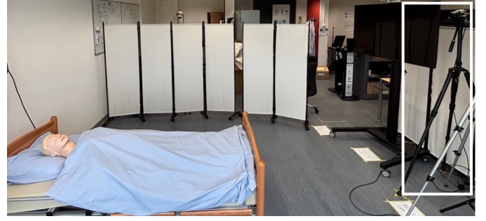
Figure 3: The setup in the Philips lab with a camera on a tripod (in the white square) and the respiration simulator underneath a sheet.
