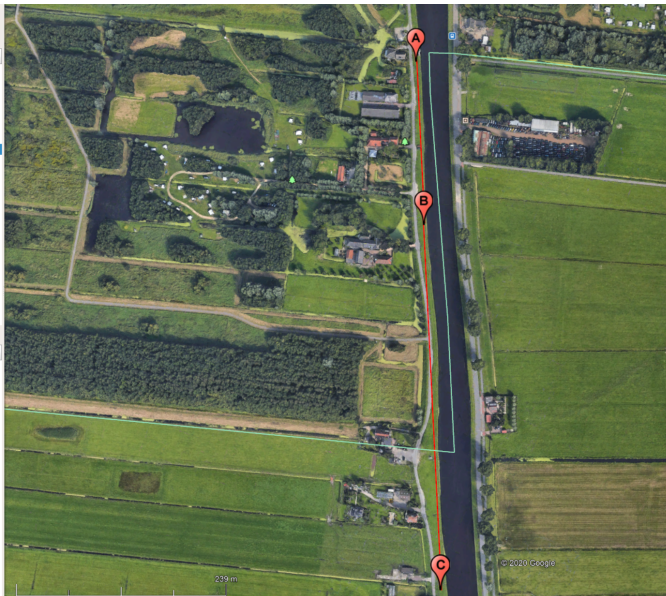
Figure 5.3: An image of the case study regional dike segment near Delft. The figure is generated using Google Earth pro. A red line drawn along the area shows where vegetation is monitored; and points A, B and C represents the locations where displacements are measured.
