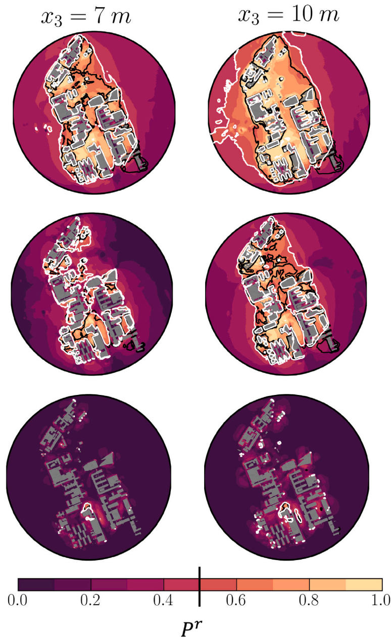
Fig. A.13. Comparison of the risk map for varying values of \alpha and \beta parameters starting. The black solid lines correspond to LoD 1.2, and the white solid lines correspond to LoD 2.2. The colours mark the risk map associated with LoD 2.2, while the grey region corresponds to LoD 1.2. Top row corresponds to \alpha = 0.03 and \beta = 0.05 , middle row corresponds to \alpha = 0.04 and \beta = 0.06 , while the bottom row corresponds to \alpha = 0.05 and \beta = 0.09 , respectively.
