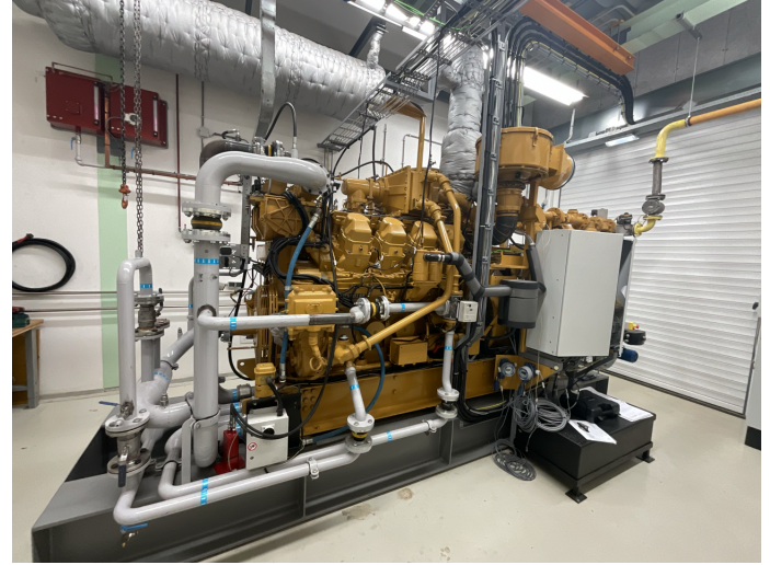
FIGURE 1: IMAGE OF THE MARINE FOUR-STROKE SPARK IGNITION ENGINE IN LAB
