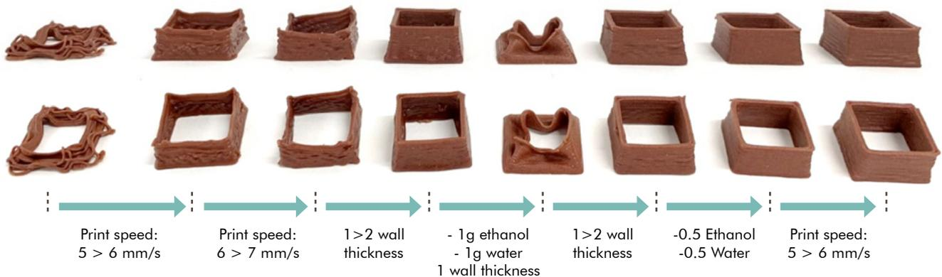
Figure 41: CL-based recipe samples with improvement in shape fidelity when print speed is increased.
