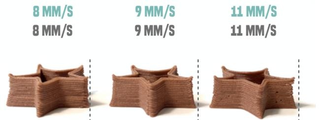
Even though AB1 displayed excellent quality at high speeds during optimization step 1, it is important to note that printing sharp corners at this speed can lead to reduced quality. When printing models with corners sharper than 90°, it is necessary to lower the print speed.
