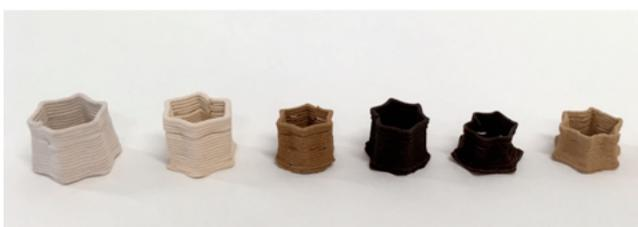
However, it should be noted that these prints did display significant shrinkage, with a 26% reduction in height and a 12% reduction in line width.
