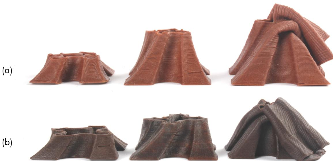
**Figure 96:** Vase shape with converging and diverging overhangs printed with AB, Collapse due to weak spot in the model.
