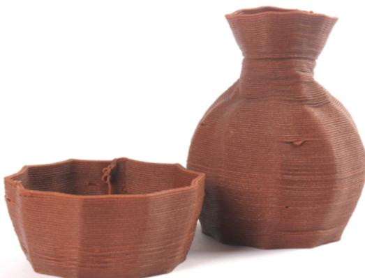
**Figure 97:** Vase shapes printed with AB1 (a) and CLAB4 (b)
