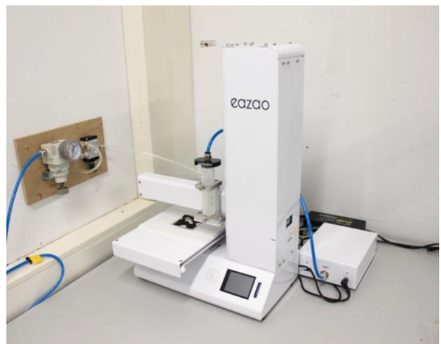
The extrusion pressure was determined separately for each print since small differences in material and environmental factors were found to influence the necessary pressure for good extrudability. The pressure was adapted until the extruded material showed no signs of under-extrusion or over-extrusion (Figure 35). The extrusion pressure was determined per recipe variation but kept constant during the printing. No fans were used while printing in this phase of the research.
